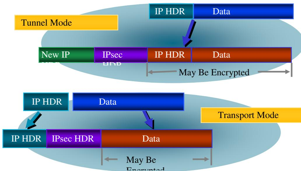
Figure 5.5: IPsec Tunnel and Transport Mode (from Cisco)
