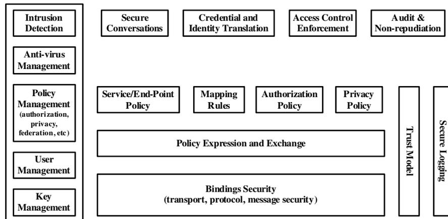
Figure 4.2: Components of the OGSA Security Model
