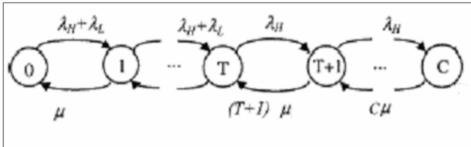
Figure 7.7 SIDM admission Model (UMTS, WLAN to WiMax)
