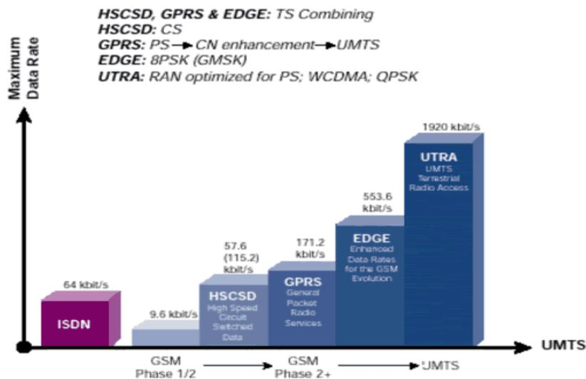
The first digital cellular system, the GSM offered a data rate of 9.6 Kbps knowing that the access scheme applied was a combination of FDMA and TDMA. Further technical
