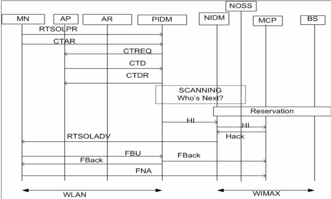
Figure 7.3 Handover from WLAN to WiMax
