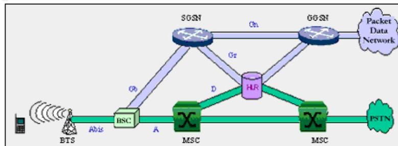
Figure 2.3 GSM/GPRS Network
