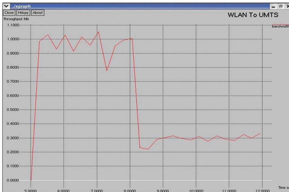
Figure 4.8 Throughput performance (WLAN/UMTS, using mipv6)
