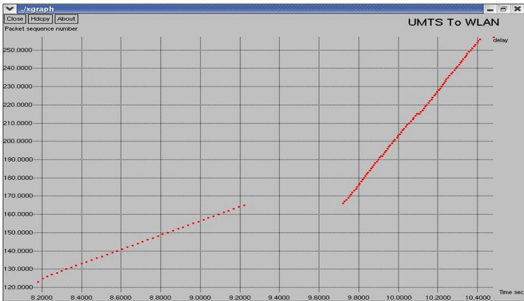
Figure 4.2: Packet sequence number Vs time using MIPv6
