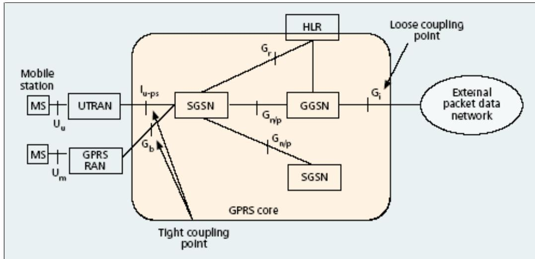
Figure 3.1 Loose and tight coupling.
