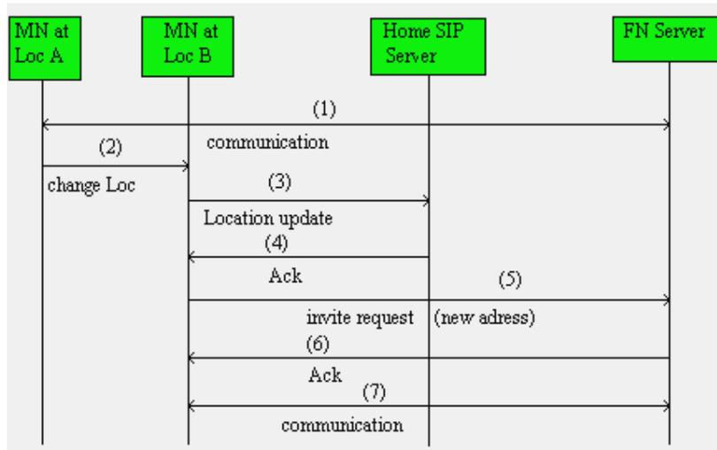
Figure 3.5 Signaling for SIP connection initialization
