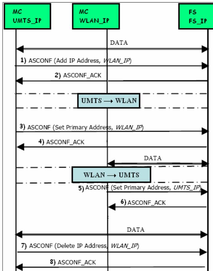
Figure 3.4 Signaling exchange for mSCTP
