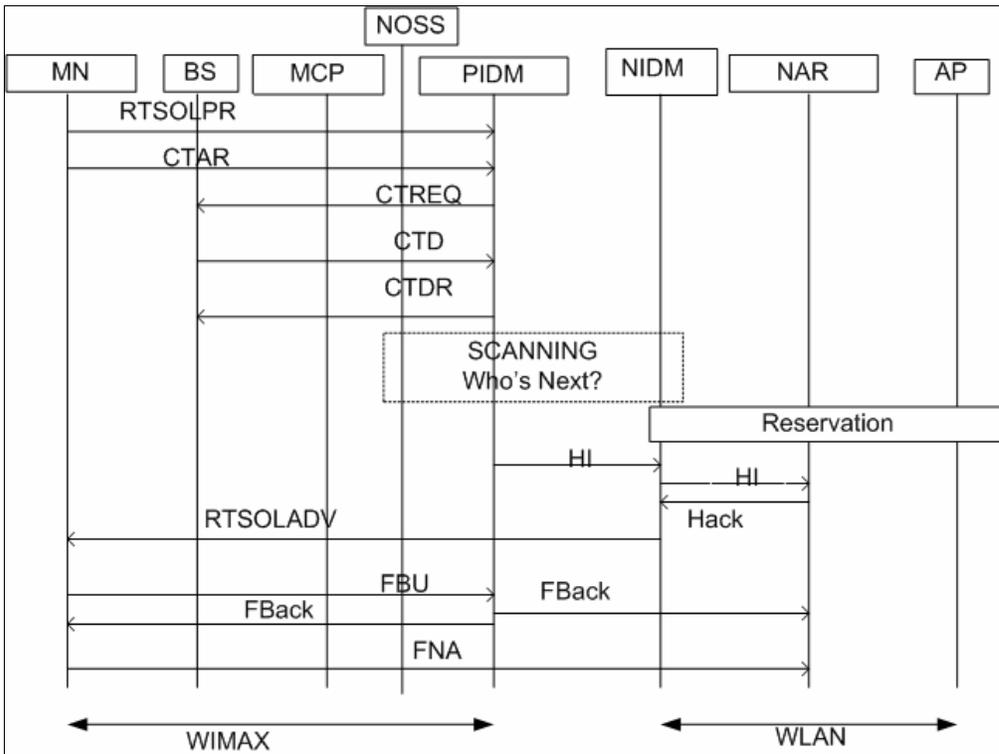
Figure 7.6 Handover from WiMax to WLAN
