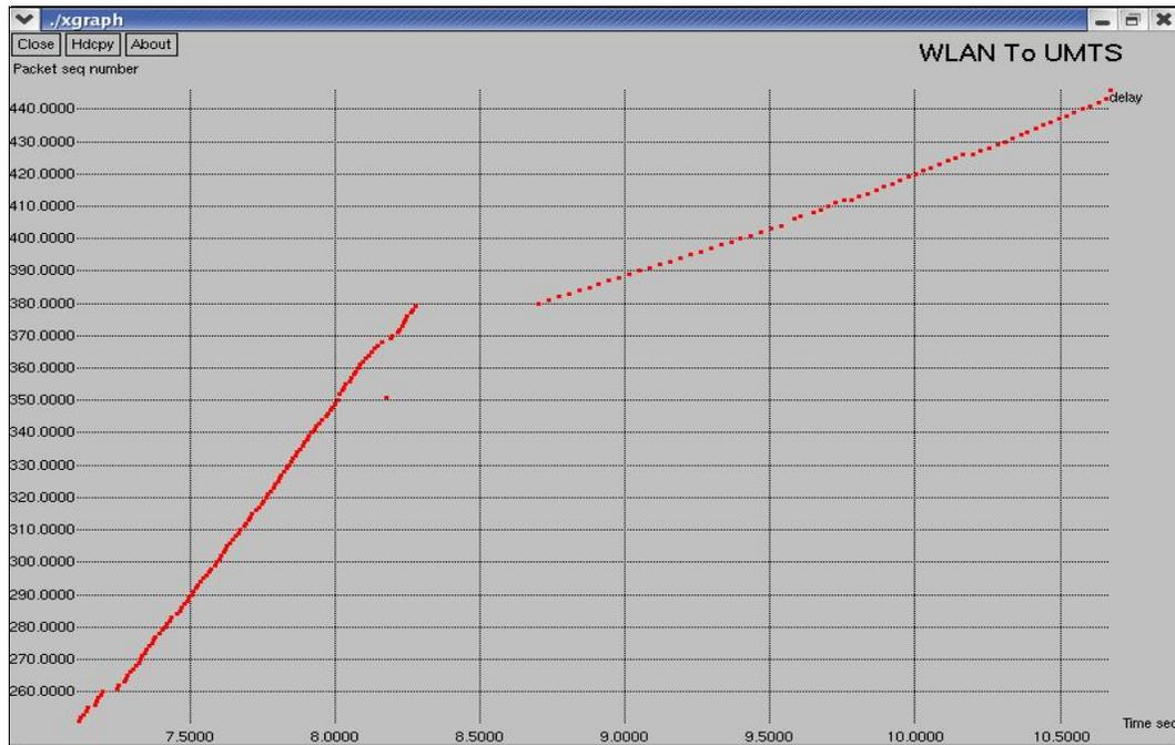
Figure 4.6 Packet sequence number Vs time with MIPv6
