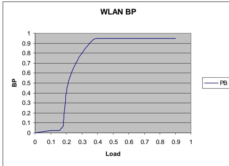
Figure 5.7 Blocking probability in function of IDM load (WLAN)
