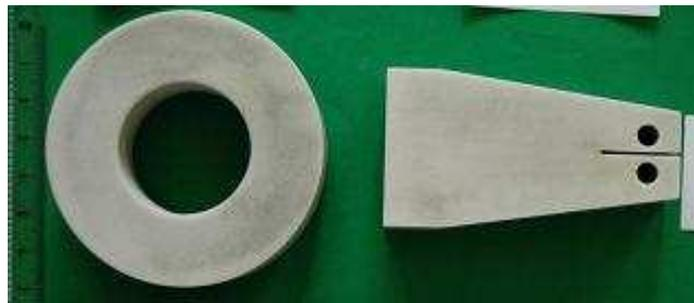
Figure 3.1: Two samples that have been used to generate fracture surfaces of glass ceramics: Modified Brazilian test geometry that leads to rapid mode I fracture (left) and modified Tapered Double Cantilever Beam geometry that leads to stable mode I fracture (right). The outside diameter of the annular sample is 80 mm.
