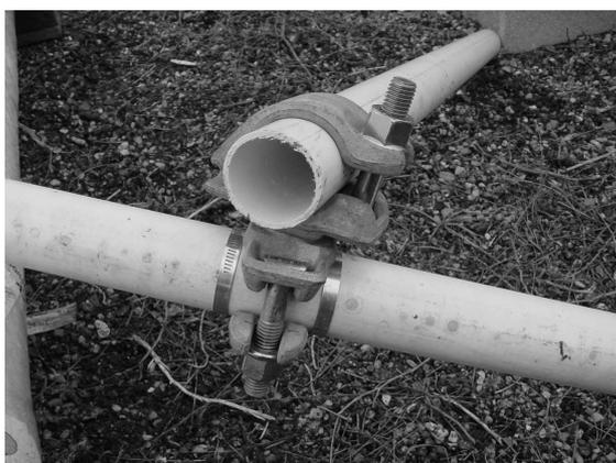
FIG. 3.11 – Assemblage orientable.
