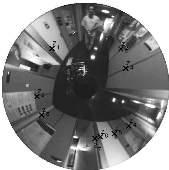
Figure 9.24: Matched points between image 640 and 645 without angular boundaries
