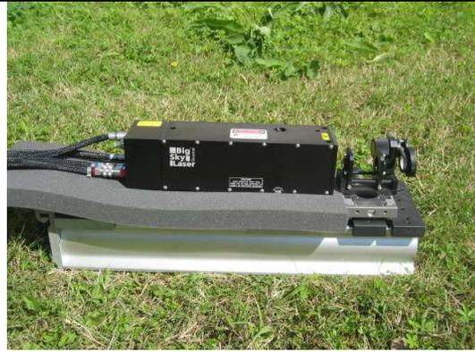
figure II-4 : Tête laser Quantel Big Sky CFR 200
