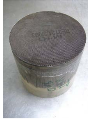
(b) DOC used with Renault M9R 2.0-L engine. 2.21-L / Ø 5.67 x 5.5 in / cell density: 400 cpsi
