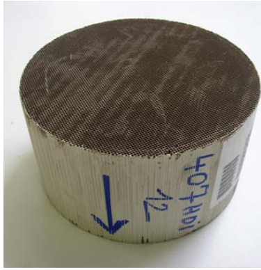
(a) DOC used with a Peugeot 407 HDi DPF 2.0-L engine. 1.22-L / Ø 5.63 x 3 in / cell density: 400 cpsi
