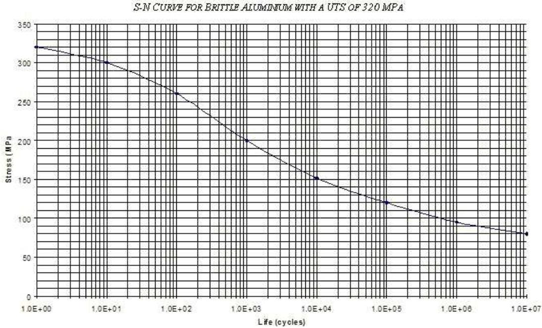
Figure 7.2: Typical example of Wöhler curve
