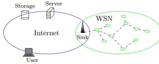
Figure 1.2: Fixed sink wireless sensor network.
