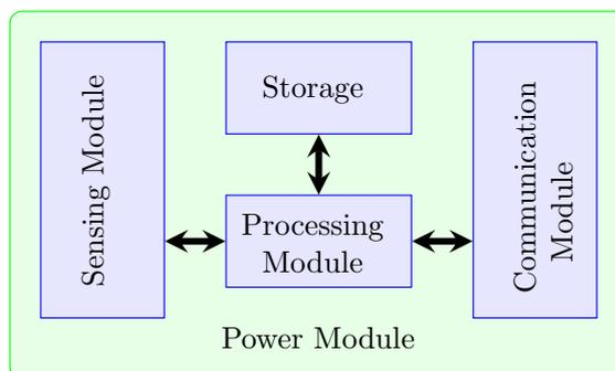
Figure 1.1: Sensor node components.
