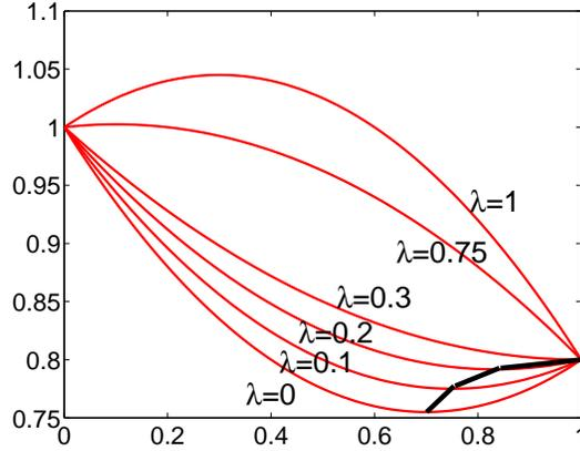
Figure 2.3: Illustration for path optimization approach.  $F_0$  ( $\lambda = 0$ ) — initial convex function,  $F_1$  ( $\lambda = 1$ ) — initial concave function, bold black line — path of function minima  $P^*(\lambda)$  ( $\lambda = 0 \dots 0.1 \dots 0.2 \dots 0.3 \dots 0.75 \dots 1$ )
