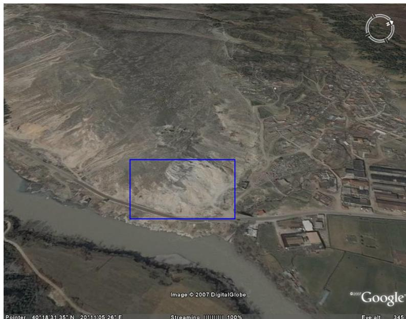
Figure 5.3. Satellite image of the studied area; the quarry is indicated by a blue square (from Google Earth 4.3, 2007). The scale of the quarry is of 70m in height and about 120m long.
