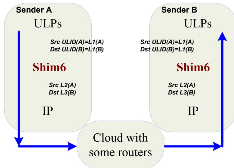
Figure 2- 7 Mapping with changing locators in shim6.
