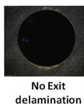
Figure 7. Performance of Reference D in Ti6Al4V-CFRP stacks
