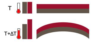
Fig. 2.13: Thermoelastic bending of a bilayer structure under heating
