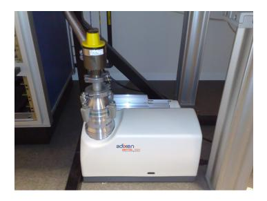
Fig. 3.18: The Adixen turbo pump used for creating the vacuum into the chamber
