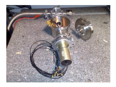
Fig. 3.16: The vacum chamber setup used for low pressure measurements
