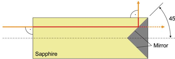
Figure C.7: Schematic beam path in the sapphire probe.
