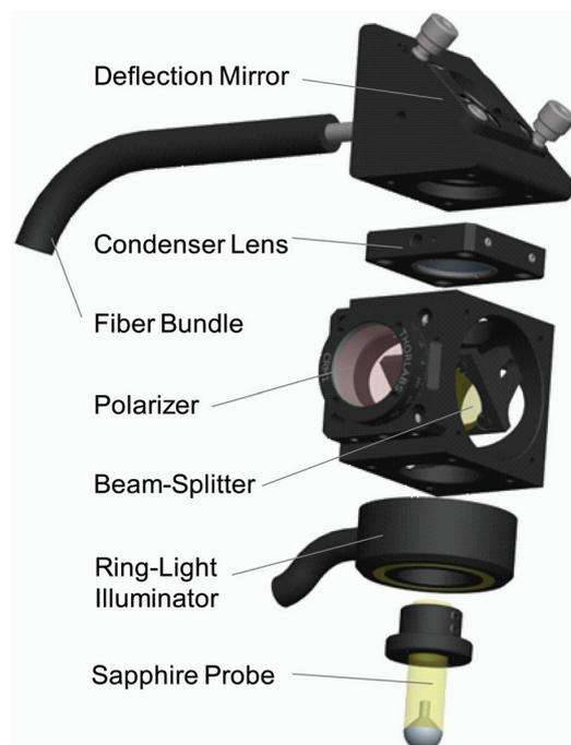
Figure C.3: Detail view of the MGI setup. The beam-splitter cube, sapphire probe and the functional components of the illumination systems are shown. Mechanical supports are not shown in the figure. The orientation is such that the camera can look through the polarizer into the beam-splitter cube.
