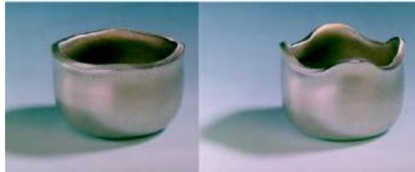
Fig. 1.2: Earing in aluminum cans [AluMATTER, 2009]
