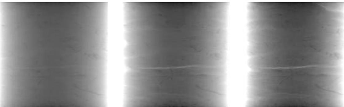
Series 6: specimen #19 in a 1,3 molar NaCl solution, immediately after the filling, after 16 minutes and before the sample failed after 45 minutes. The whole sample is full of many cracks, growing from the surface towards the centre of the sample. Load =1.5 MPa, T =25°C, picture width = 16mm,  $\mu\text{CR}=22\mu\text{m}$ .
