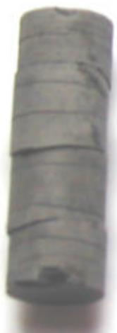
Figure 33: exhibits strong fissuring in the bedding plane of a shale sample from the site of Est, after immersing into a 2 molar KCl solution. The specimen is a cylinder with 16mm in diameter and a height of 30 mm.
