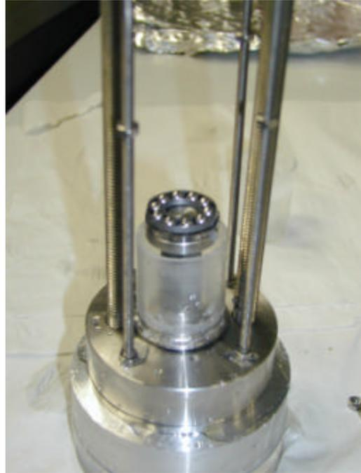
Figure 68: Device during preparation before a test with a solution (empty reservoir with sample and upper bearing).
