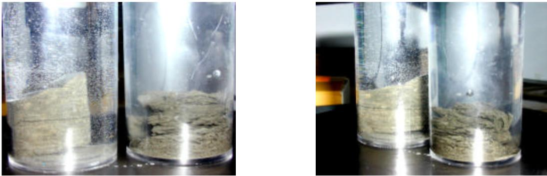
Figure 74 a), b): The left glass contains a 1.3 molar KCL solution. The other cylinder is filled with pure water  $G=56$  nS. The KCL glass is completely covered with small gas bubbles and the sample does not disperse but cracked. Both glasses contain material from sample #05564, well 205.
