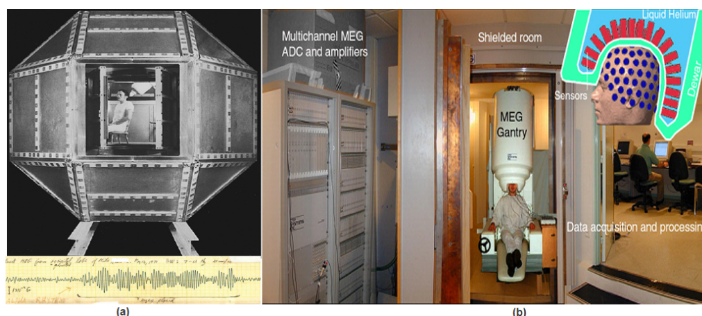
Figure 3: (a) First MEG recording at MIT inside a spaceship like magnetic shielded room using single channel SQUID. (b) MEG Setup at La Pitié-Salpêtrière Hospital, Paris inside modern multilayer shielded room using 151 SQUIDs covering whole brain.
