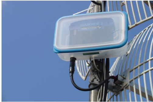
(a) Initially, simple Tupperware has been used to protect the routers
