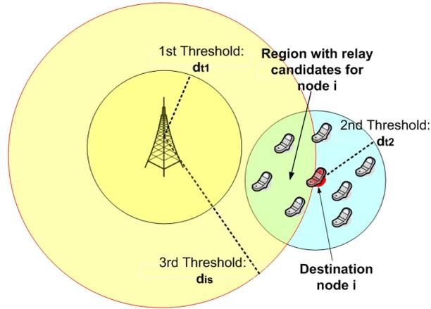
Figure 6.7: The proposed relay selection technique (Algorithm 6). 3 thresholds are employed for determining the relay candidates for target node  $i$ :  $d_{t1}$ ,  $d_{t2}$  and  $d_{is}$ .
