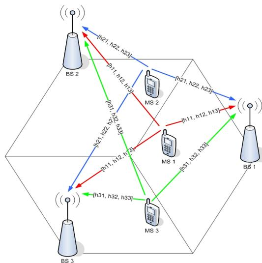
Figure 4.3: Phase 2 of the proposed decentralized MCP framework.
