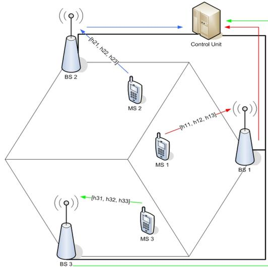
Figure 4.1: Phase 2 of the typical centralized MCP framework.
