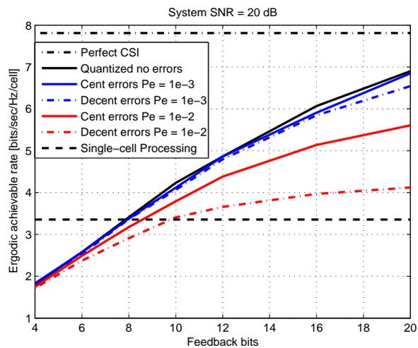
Figure 4.9: *Digital Feedback*: Sum-rate versus the number of feedback bits (System SNR = 20 dB). Blue curves:  $P_e = 10^{-3}$ , Red curves:  $P_e = 10^{-2}$ . 'Cent': centralized framework, 'Decent': decentralized framework.
