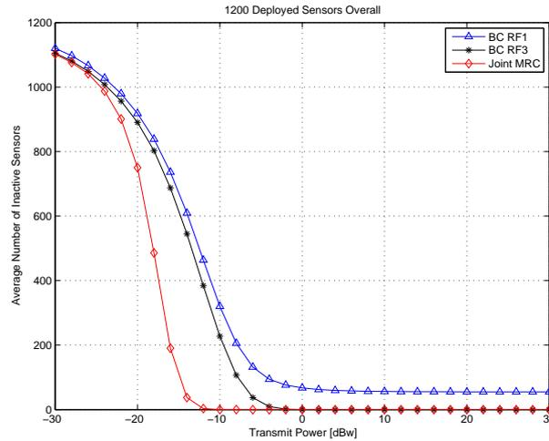
Figure 7.2: Average Number of Inactive Sensors vs. TransmitPower.
