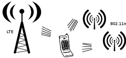
Figure 8.1: Dual-mode receiver scenario.
