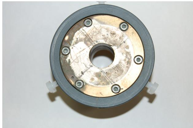
Figure 4.3: Picture of the fabricated current monitor.
