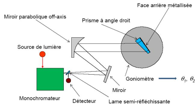
Figure III - 5 : Configuration de Littrow.
