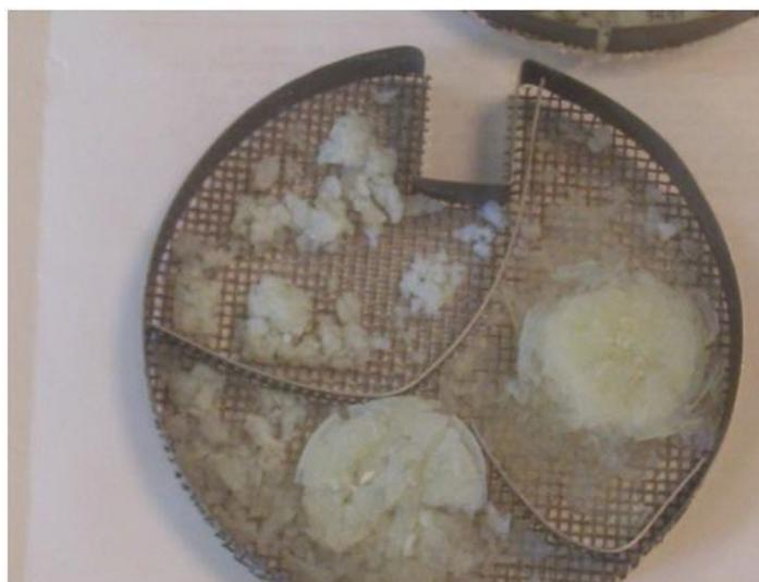
**Figure. 2.46.** Example of  $\text{TiO}_2$  aerogels obtained according to our elaboration process (diameter of the grid is around 9 cm)
