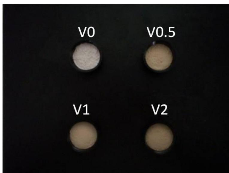
Figure 3.2: Color change of vanadium doped nanotubes
