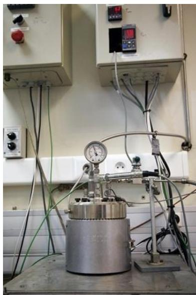
Figure 2.45. Photography of the autoclave used for supercritical  $\text{CO}_2$  drying
