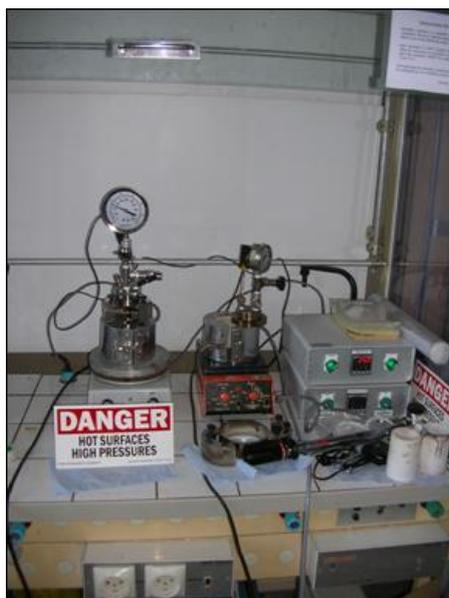
**Figure 2.3 Autoclave for hydrothermal crystallization**
