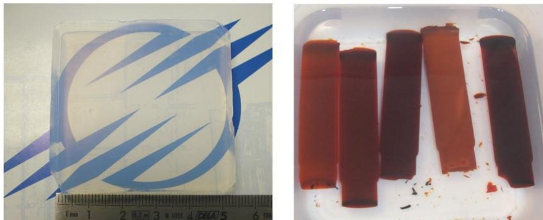
**Figure 1.24. Examples of mineral aerogels and organic gels. Left : monolithic silica aerogels issued from supercritical drying [Masmoudi, 20062006]; right : resorcinol-formaldehyde based-gels (private collection of Dr. Sandrine Berthon-Fabry, MINES ParisTech, CEP, Sophia Antipolis, France)**
