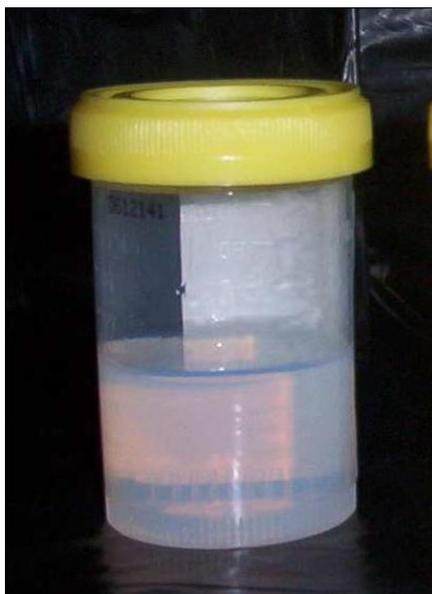
**Figure 2.44** Example of a TiO<sub>2</sub> gel synthesized according to our sol-gel route
