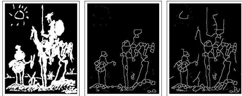
(a) 2D binary image. (b) Skeleton of (a) with no constraint (c) Skeleton of (a) where end points of the initial image have been preserved.
