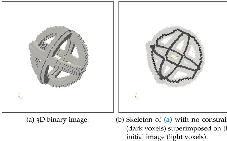
Figure 17: Computation of the skeleton of a 3D binary regular image.
