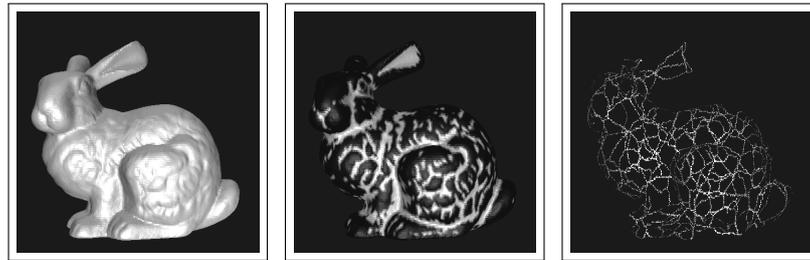
(a) Triangle mesh surface. (b) Surface curvature. (c) Surface skeleton.
