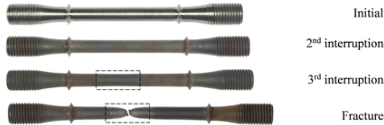
Figure 3.11: Evolution of necking during creep at 350 MPa and 500°C.
