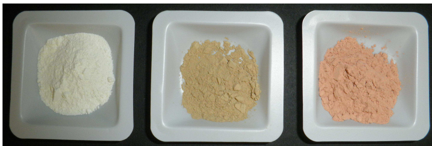
Figure 1.1: Photograph of bulk \text{GdVO}_4 powder from different synthesis methods. Samples were obtained from coprecipitation at room temperature (left, sample MS20), from coprecipitation and subsequent thermal treatment at 900^\circ\text{C} (middle, MS11) and from the ceramic method at 1250^\circ\text{C} (right, MS8).
