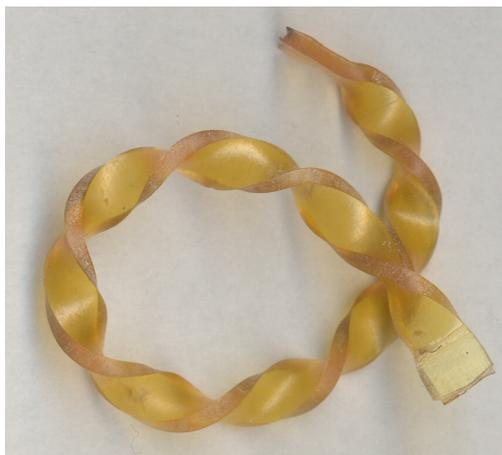
Figure 15 – The equilibrated torsade is bent into a loop at 100 °C and cooled down below T<sub>g</sub>. If we heat it up above T<sub>g</sub> again, it will retrieve its straight twisted shape.
