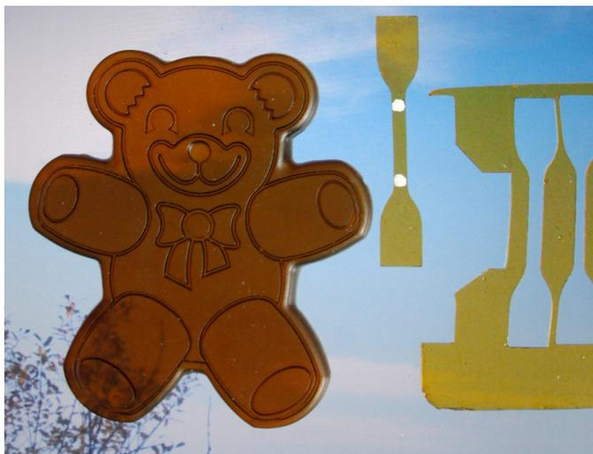
Figure 4 - Large transparent defect-free articles obtained by molding and punching.
