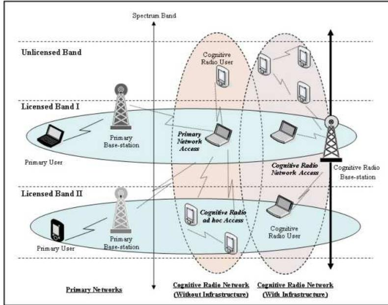
Figure 3.1: Architecture of Next Generation Wireless Networks [3]
