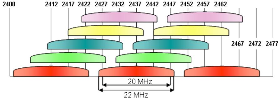
Figure 4.1: IEEE 802.11b channelization scheme (figure inspired from [13])
