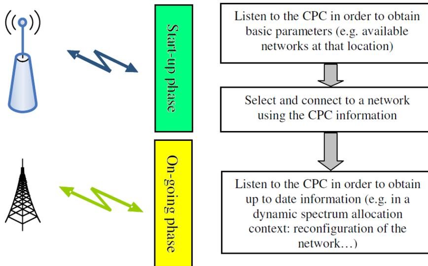
Figure 5.5: CPC capturing procedure (figure inspired from [50])
