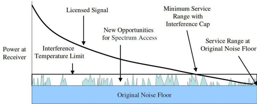
Figure 3.3: Interference Temperature model [23].
