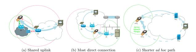
**Figure 3.3** Typical use-case scenarios of a multihomed mobile device: (a) Public Wi-Fi provisioned with a 3G uplink (*e.g.*, commuter train or ferry); (b) Data server on a network offering wireless access but a slow uplink; (c) 802.11 *ad hoc* link is available which is much shorter than going through both HAs or even the infrastructure.
