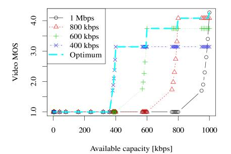
Figure 3.11 Quality profiles (2.5) for a video stream encoded with H.264 at various rates for varying network capacities. The optimum MOS is not a linear function of the available capacity. At a chosen bit-rate, a reduction in capacity may make no difference or may make the video unusable.
