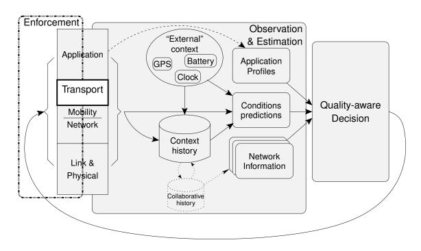
Figure 4.2 Relation of the contribution presented in this chapter to the cross-layer framework of this thesis. Bold lines and non greyed-out components are the current focus.
