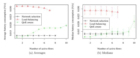
Figure 3.14 Battery consumption depending on the number of active flows for each approach. A consumption of 0.03%/s results in a battery lifetime of less than an hour. The apparent decrease in consumption of the load-balancing strategy is biased by the limited number of scenarios with 8 or more flows which could run without hitting the time limit.
