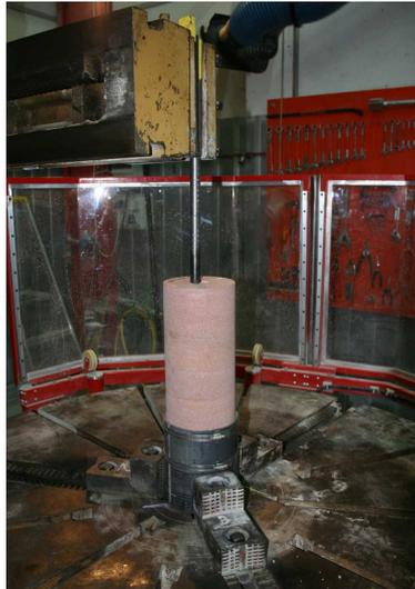
(a) overview of the vertical lathe during the rifling of a borehole.
