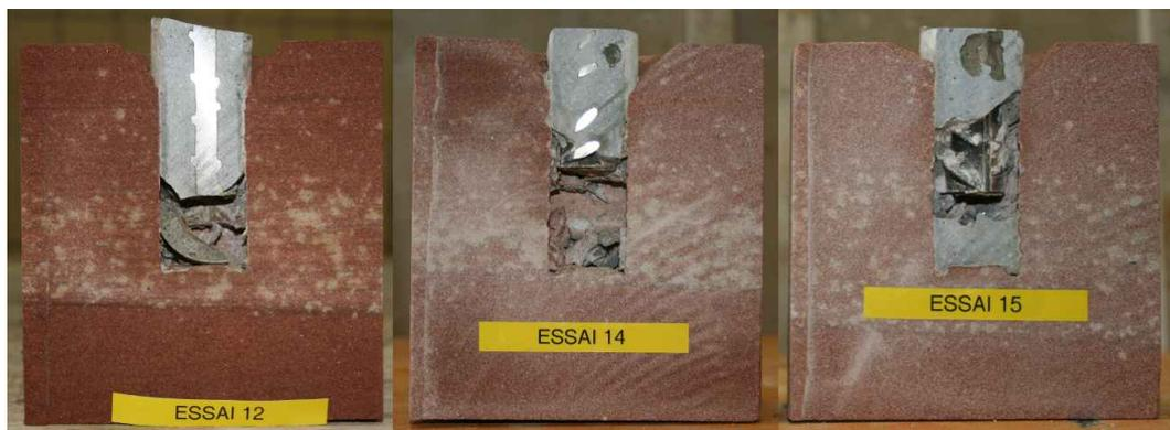
**Figure A.7:** Openview of the tests 12, 14 and 15 samples.
