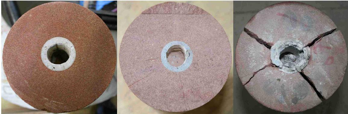
**Figure 3.17:** aspect of the grout and rock annuli after three pull-out tests conducted on HA25 rockbolts at constant  $p_r$ . From left to right:  $p_r = 10$  MPa,  $p_r = 5$  MPa and  $p_r = 1.2$  MPa.
