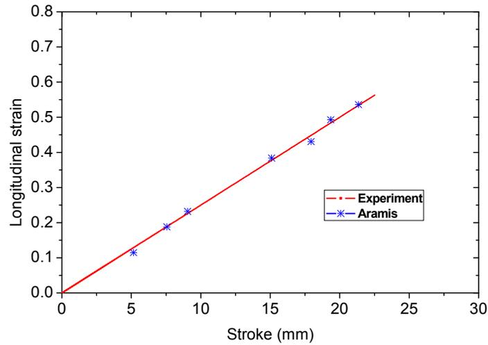
Fig.11 Comparison between the strains measured from the tensile set-up and ARAMIS system (200<sup>0</sup>C, 0.01s<sup>-1</sup>)
