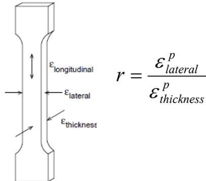
Fig.12. Definition of Lankford coefficients in the test [8]
