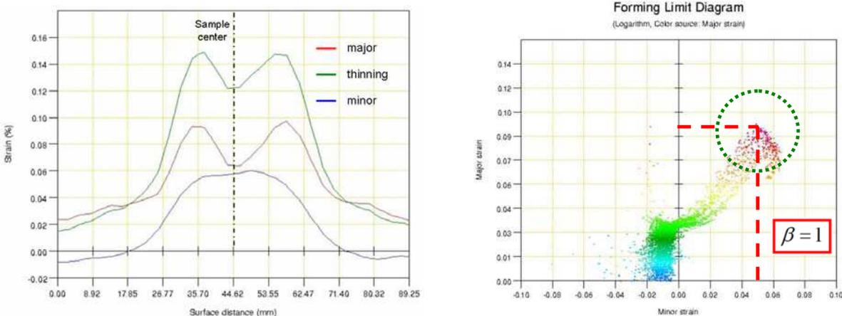
Fig.14. Major and thinning strains and Forming Limit Diagram (FLD) given by ARAMIS (100<sup>0</sup>C, safe specimen)
