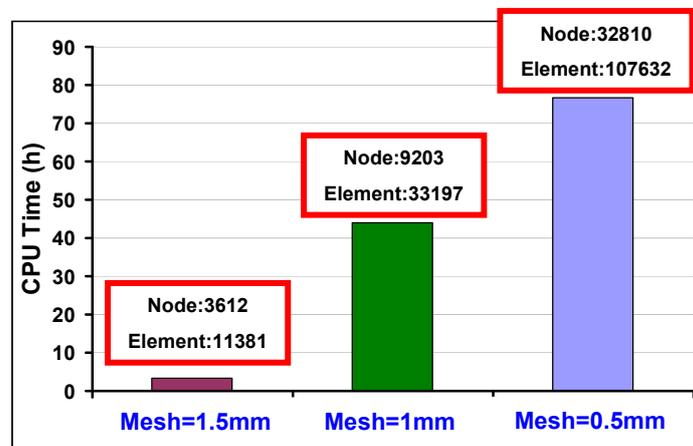
Fig.25. The CPU time with various mesh size.
