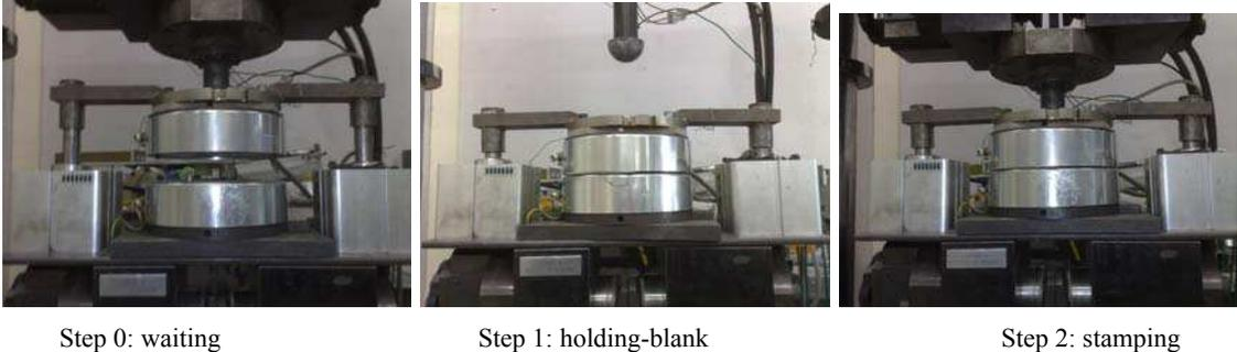
Fig.2. The procedure of the Nakazima stamping tests
