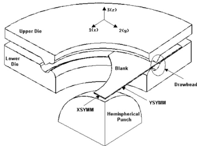
Fig.4. The modeling layout of Nakazima test [14]
