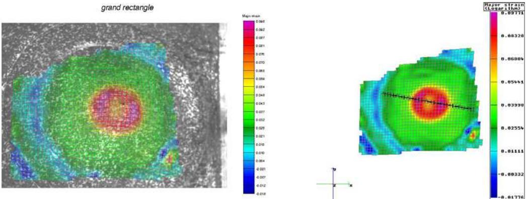
Fig.13. The strain measurements in blank diagonal section (100<sup>0</sup>C, safe specimen)
