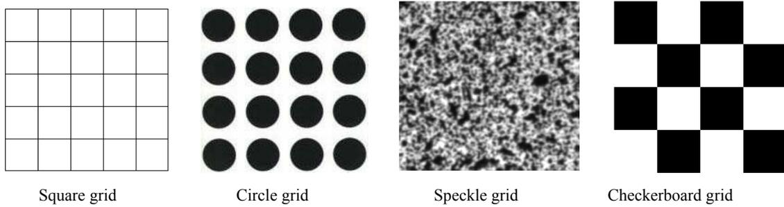
Fig.5. Different patterns used by optical measurement systems
