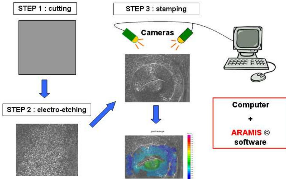
Fig.6. The ARAMIS system operate procedure
