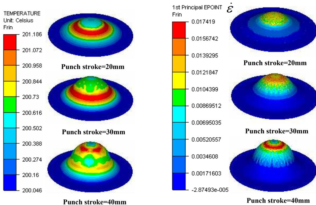
Fig.9. Result of numerical simulation for different punch strokes (FORGE).
