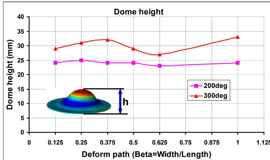
Fig.18. Dome - height for various strain paths.
