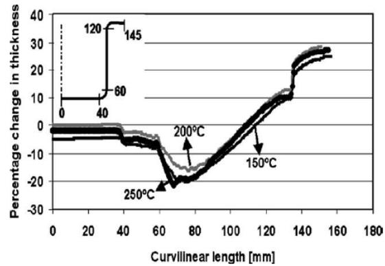
Fig.14. Thickness distribution for LDR of 2.3 [11].
