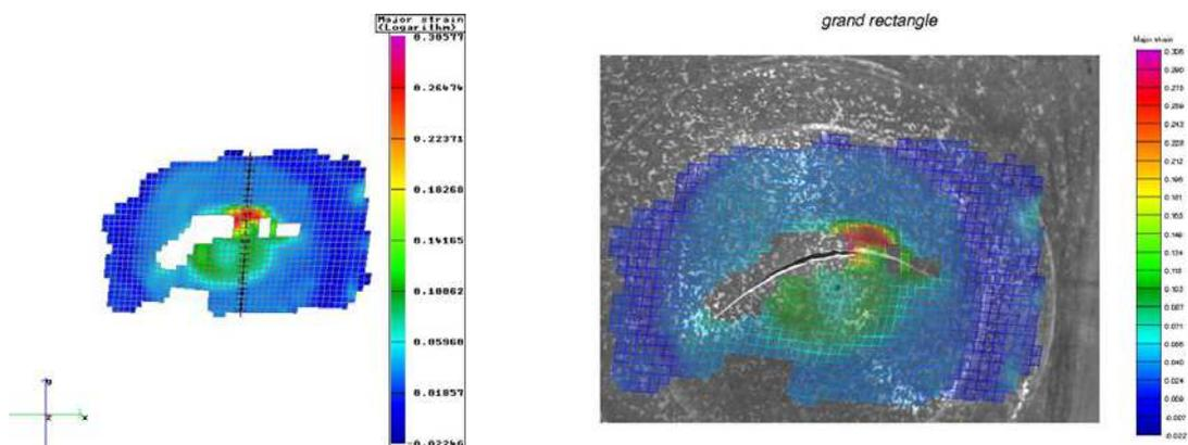
Fig.12. Strain distribution measured by ARAMIS (100<sup>0</sup>C)
