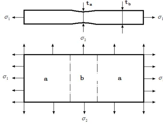
Fig. 24. Simple schematic diagram of M-K analysis.
