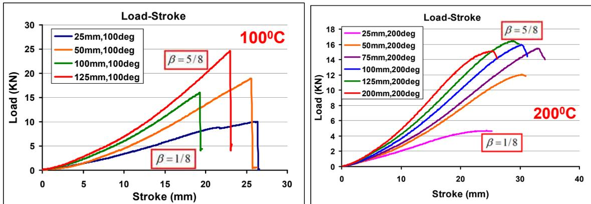
Fig.21. Load - stroke curve at various blank widths.
