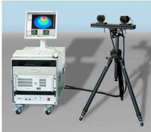
Fig.9. The ARAMIS measurement system set-up in laboratory
