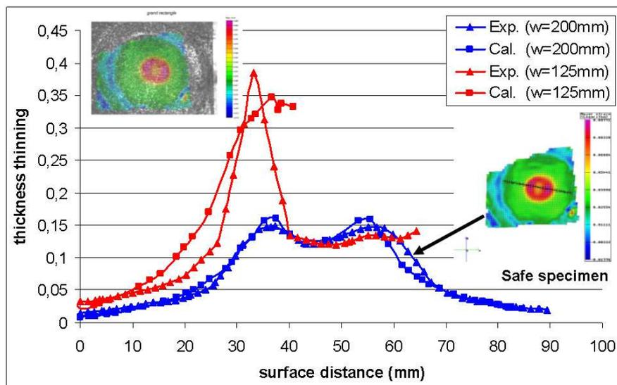
Fig.11. Thickness distribution from simulation and experiment at 100<sup>0</sup>C (FORGE).
