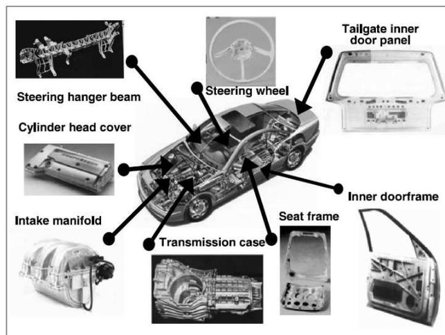
Fig.16. Application of magnesium alloys in motor vehicles [37].
