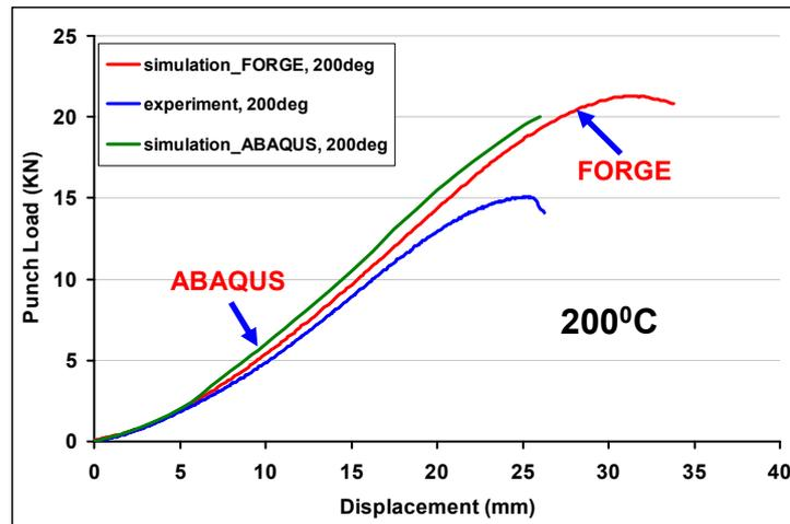
Fig.14. The comparison of punch load in FROGE and ABAQUS.
