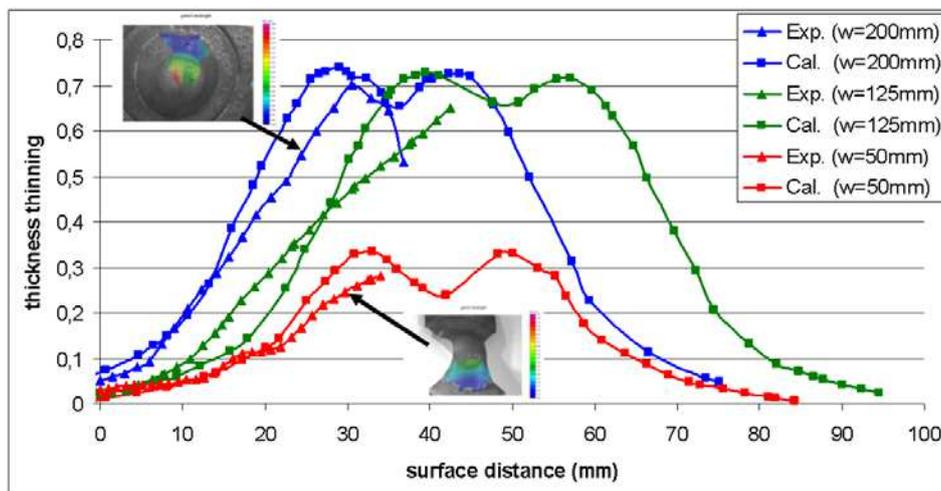
Fig.12. Thickness distribution from simulation and experiment at 200<sup>0</sup>C (FORGE).
