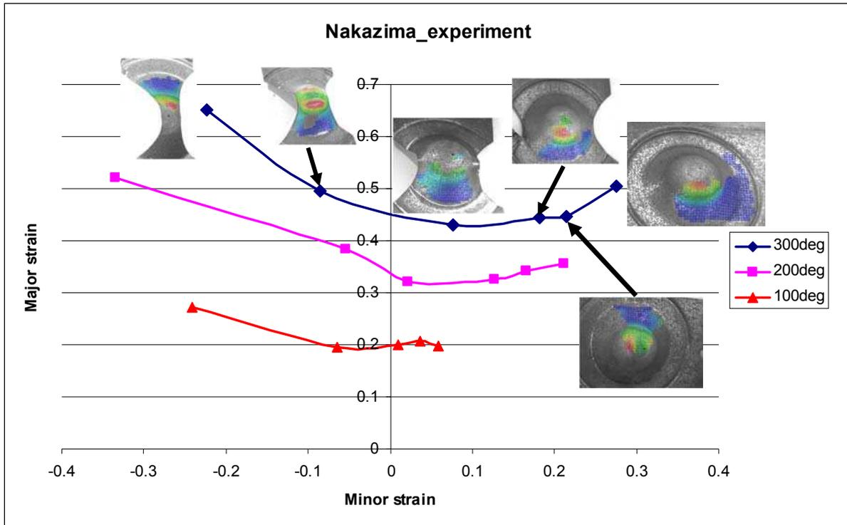
Fig.15. Broken FLD identified by Nakazima experiments
