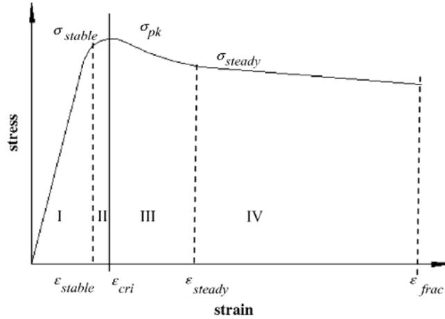
Fig.10. Typical flow stress curve at the elevated temperature for HCP structural material [26].
