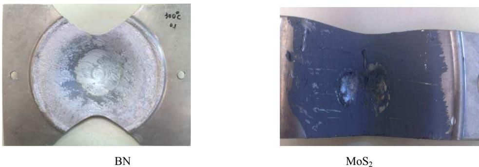
Fig.23. Warm stamped specimens with two different lubricants.
