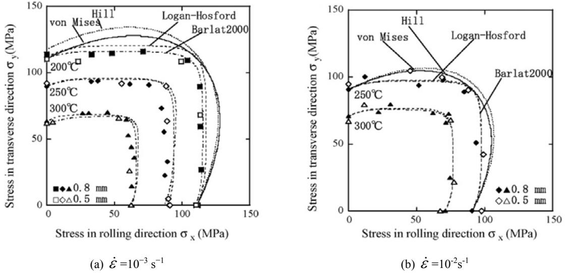
Fig.9. Comparison of experimentally obtained yield loci of Mg alloy sheet with those predicted by the von Mises, Hill, Logan-Hosford and Barlat criteria ( $t_0 = 0.8$  and  $0.5\text{mm}$ ) [22].
