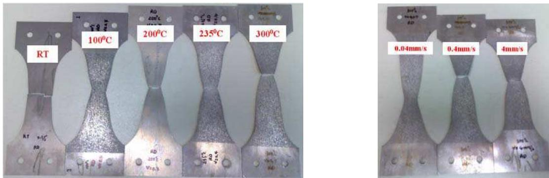
(a) Specimens at various temperatures ( $v=0.4\text{mm/s}$ , RD)
