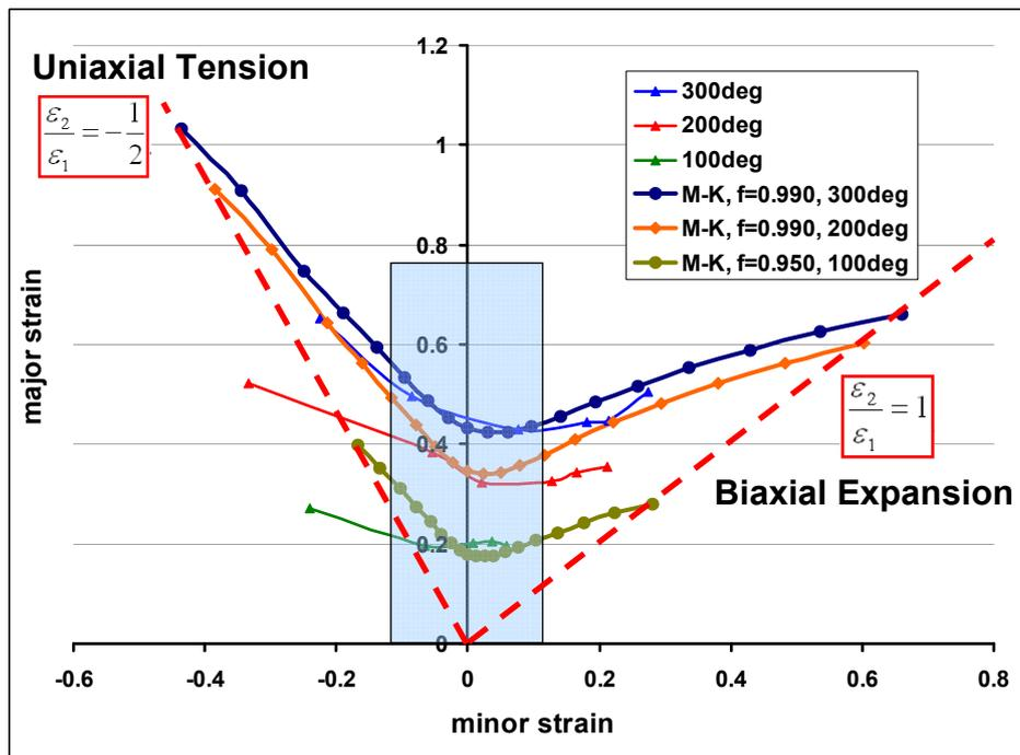
Fig.26. M-K prediction and experiment FLD comparison
