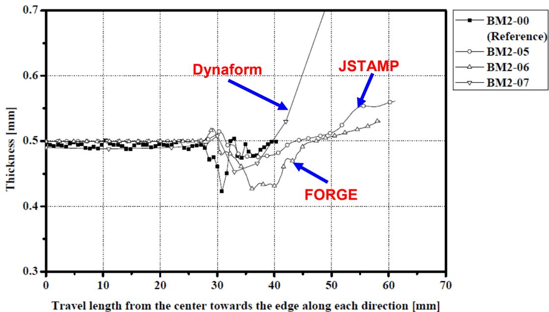
Fig.30. Thickness vs. Travel length from the center toward the edge [27].
