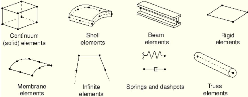
Fig.1. Finite element families used in analysis [6].
