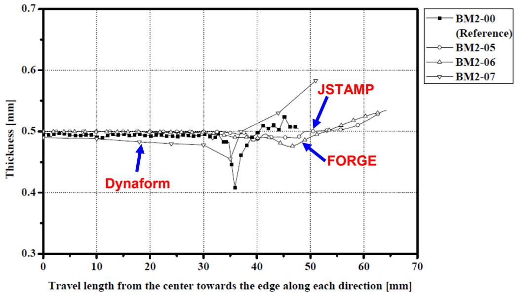
Fig.29. Thickness vs. Travel length from the center toward the edge [27].
