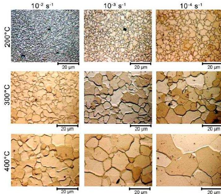
Fig.4. Optical micrographs specimens illustrating the DRX microstructure under uniaxial compression at various deformation conditions ranging from 200 to 400°C and  $10^{-2}$  to  $10^{-4} \text{ s}^{-1}$  [16].
