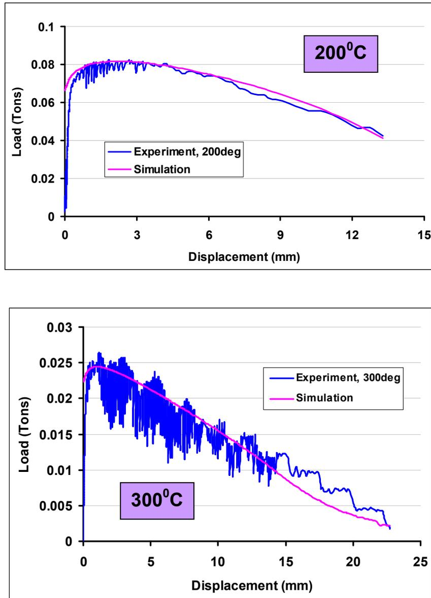
Fig.15. Comparison between experiment and simulation with Lemaitre damage model in tensile test ( $\dot{\epsilon}=0.01s^{-1}$ ).
