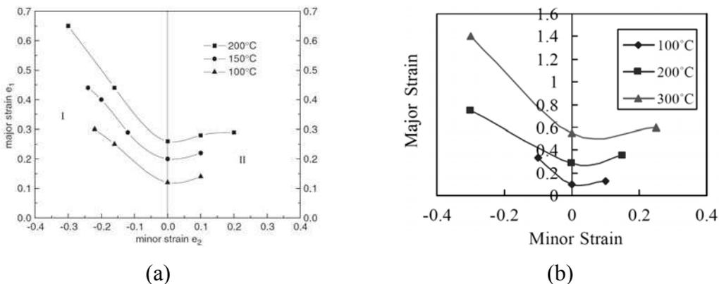
Fig.11. The forming limit diagrams at various temperature [27, 28].
