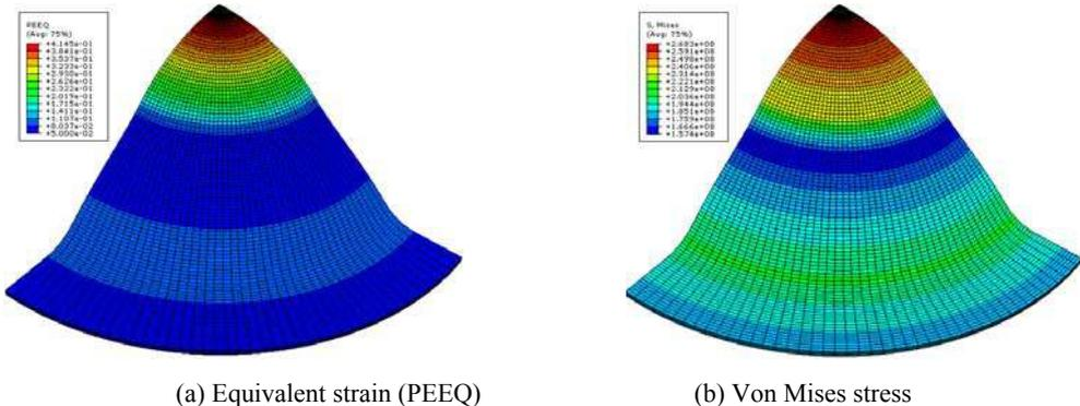
Fig.8. Distributions of equivalent strain and Von Mises stress in ABAQUS (200<sup>0</sup>C).
