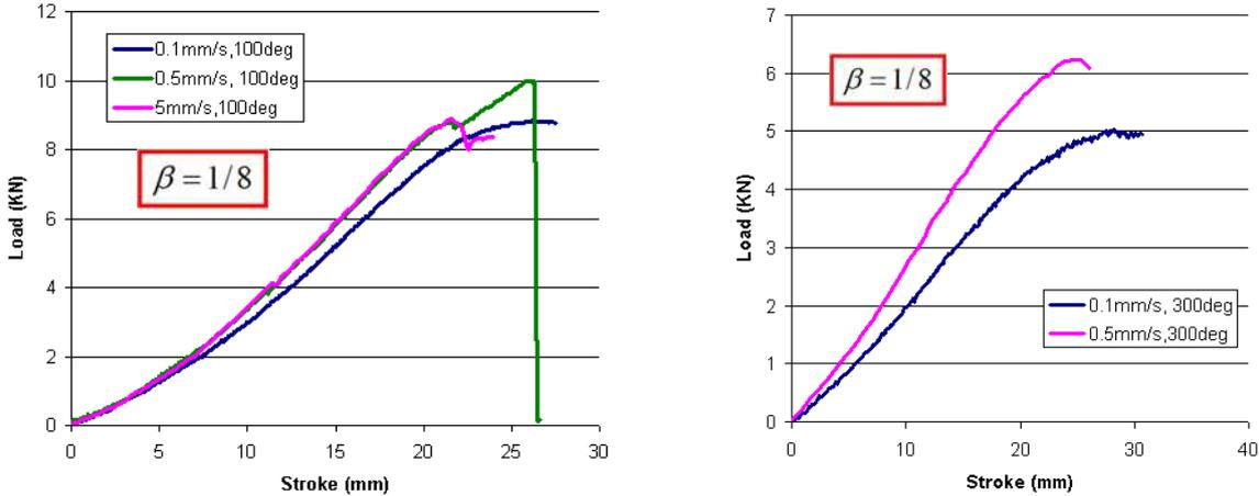
Fig.19. Load - stroke curves at various punch velocity.
