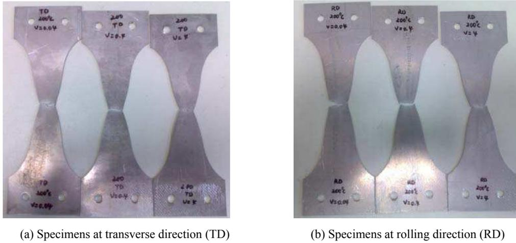
Fig.5. Deformed specimens at different forming direction (T=200°C)
