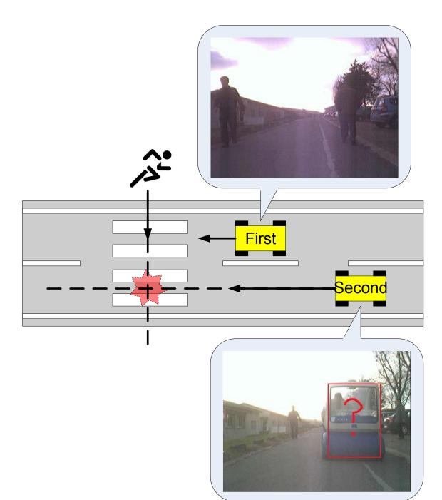
Figure 1.7 Overtaking scenario: potentially dangerous
