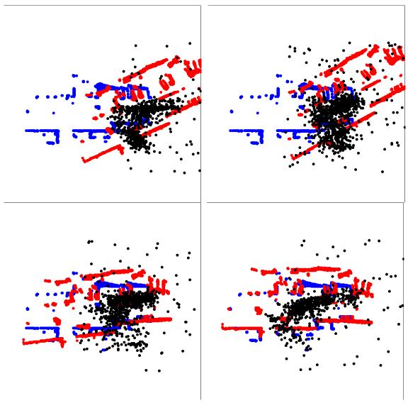
Figure 6.27 Re-convergence (or recovering) from kidnapping
