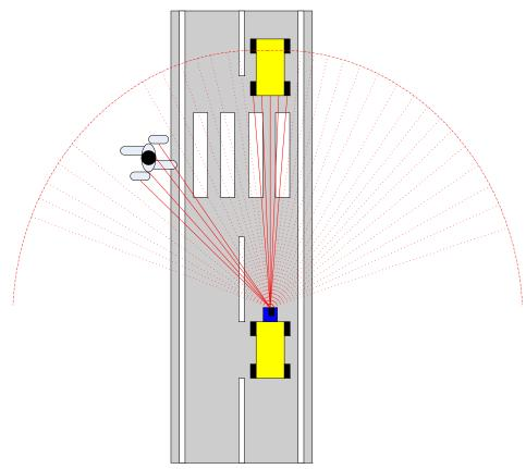
Figure 2.2 Range measurements provided by a laser scanner
