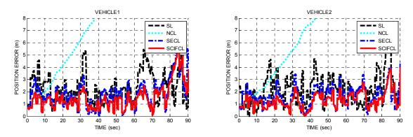
Figure 6.7 Performance of the SL method, the NCL method, the SECL method and the SCIFCL method (homogeneous absolute positioning ability)
