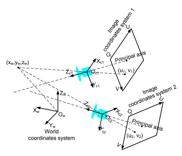
Figure 5.3 Multi-views perspective geometry
