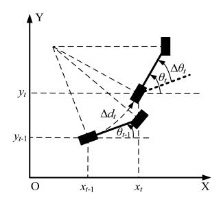
Figure 3.1 Kinematic bicycle model
