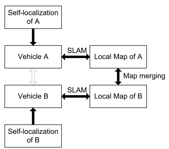
Figure 3.3 Indirect vehicle-to-vehicle relative pose estimation strategy
