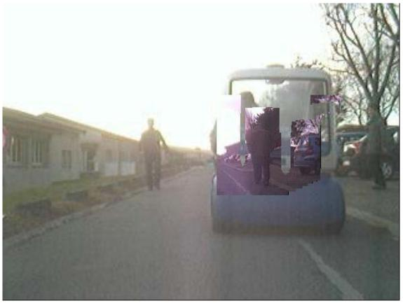
Figure 2.15 Augmented reality: 'see' through the front vehicle
