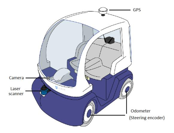
Figure 2.3 Intelligent vehicle sensor configurations (CyCab vehicle platform)
