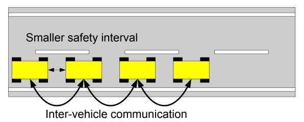
Figure 1.2 Vehicles platooning: (top) non-cooperative platooning; (bottom) cooperative platooning
