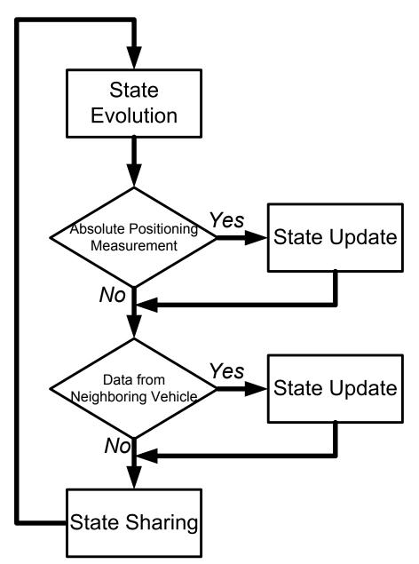
Figure 3.2 Distributed cooperative localization procedures at one vehicle
