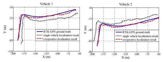
Figure 6.9 Localization results at the existence of counteracting GPS bias errors
