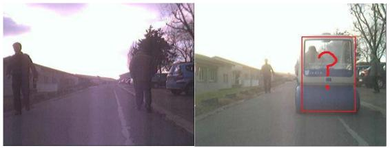
Figure 5.1 Front-following vehicles scenario: (left) the view of the front vehicle; (right) the view of the following vehicle (occluded by the front vehicle)
