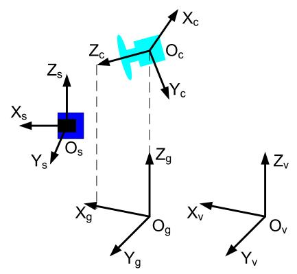
Figure 5.4 Coordinates systems in an intelligent vehicle
