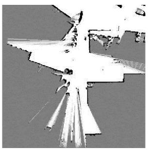
Figure 2.13 Occupancy grid based representation
