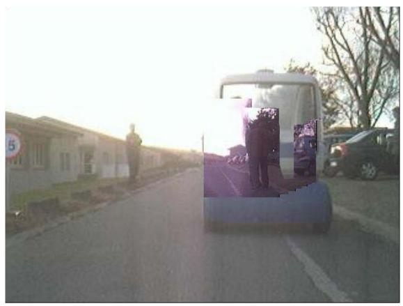
Figure 6.32 Cooperative augmented reality effect: 'see' through front vehicle
