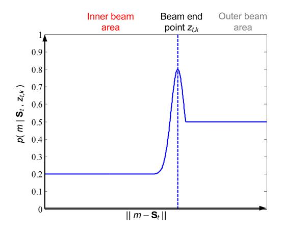
Figure 4.2 The inverse measurement model  $p(m|S_t,z_t)$
