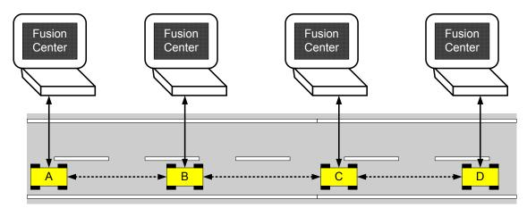
Figure 2.7 Decentralized (or distributed) operation architecture
