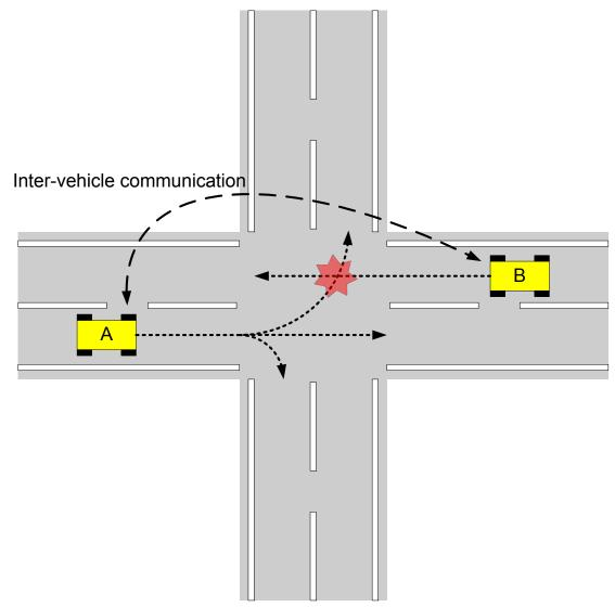
Figure 1.3 Cooperative collision warning-avoiding at an intersection
