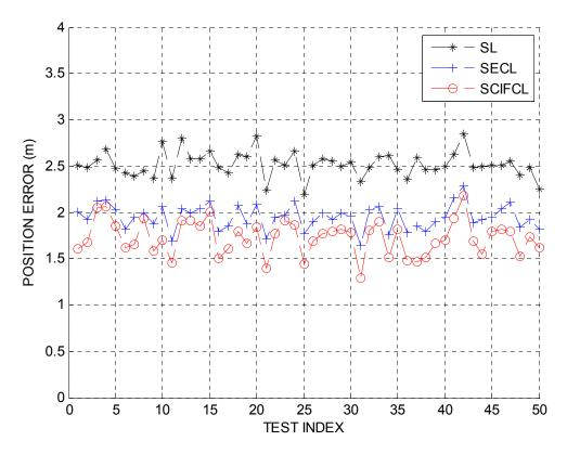
Figure 6.8 RMS of the localization error associated with the SL method, the SECL method and the SCIFCL method (homogeneous absolute positioning ability)
