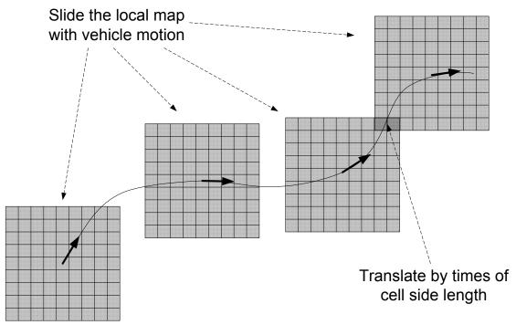
Figure 4.4 Slide the local occupancy grid map with vehicle motion
