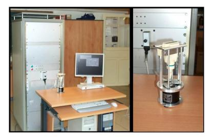
Fig 1.12. (Left) ultrafast imaging system. The electronic system composed by 128 independent channels (emission/reception), allows the acquisition of the echo-signals coming from each of the 128 elements of the probe. The entire system is controlled through a computer. (Right) The ultrasound probe (linear array) is fixed to a vibrator which excites the tissue to generate the shear waves[4].
