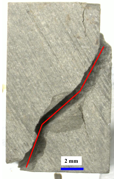
Figure 4.30: Fracture of sample in test #3 observed by optical microscopy.
