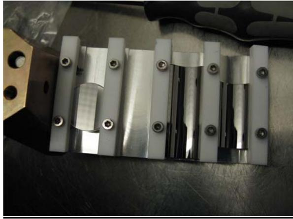
**Figure 5 :** Photo of the three mirrors (the witness on the left side and the two EHRXI mirrors) mounted in the support of the reflectometer at PTB.
