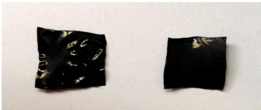
**Figure V-14** Two cellulose-CB composite film samples after drying. On the left “three-layer” route, and on the right the “mix” route.
