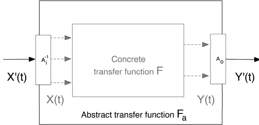
Figure 4.6: Abstraction of a transfer function
