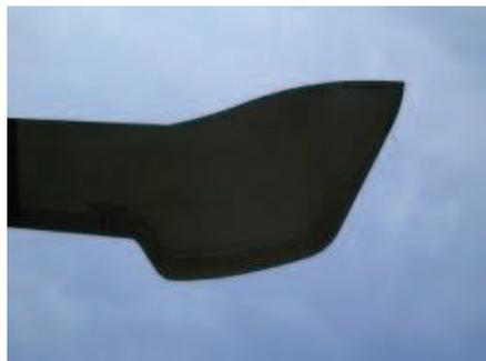
FIGURE 2.11: Pale issue de British Experimental Rotor Program
