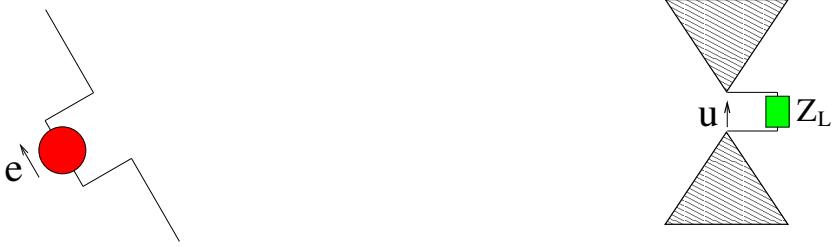
Figure 2.1: Ideal reader (left) and tag (right) antennas in LOS.
