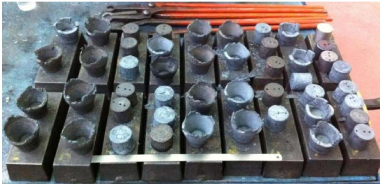
Fig. 4.1. M2 parts obtained by thixoforging process.
