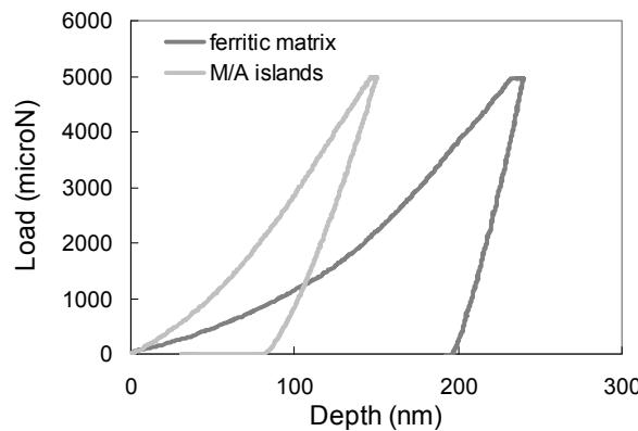
Figure I.29. Loading/ unloading cycle for Steel 1.
