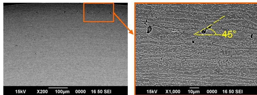
Figure III.29. SEM observations of damage at hard band located just under the outer surface (Nital etching). Bending up to 110° for thickness-reduced Steel 2.
