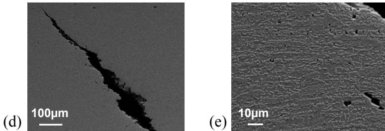
Figure 9: Fractographic observations by SEM of a broken sample after stretch bending. (a) General view with mid-thickness surrounded by a white ellipse, (b) close-up view of the mid-thickness with some of cleavage showed by white arrows, (c) close-up view of ductile failure with dimples far from the mid-thickness. (d, e) SEM observations after Nital etching of the crack and damage close to the crack at hard bands. The crack in the upper right corner of (e) is the one shown in (d).
