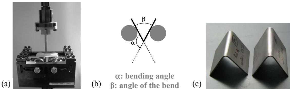
Figure I.35 : (a) Air-bending device, (b) schematic and (c) bent specimens.
