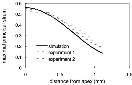
Figure 13: Evolution of the major strain at outer surface after bending up to  $180^\circ$  followed by unloading. Experimental values (strain field measurements vs. model predictions). Section taken perpendicularly to the apex at the end of the test. Curvilinear abscissa in mm along the outer surface.
