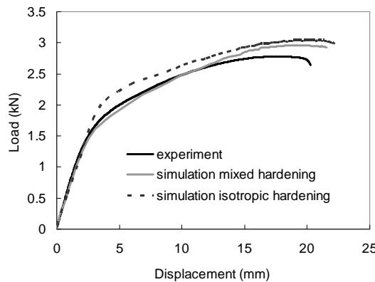
**Figure 9:** Experimental and predicted load / punch displacement curves of a prestrained and then air-bent specimen. Model predictions assuming either purely isotropic or mixed hardening rules are respectively represented with a dotted grey line and a continuous grey line.
