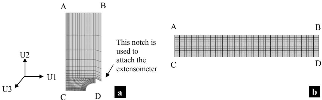
Figure 3: two-dimensional view of (a) meshing of the NT specimen (1/8 of the specimen due to symmetry with smallest element size = 130 x 150 x 800 µm close to the U-shaped notch) and (b) meshing of the shearing specimen (1/2 specimen with element size = 500 x 450 x 800 µm)
