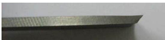
Figure I.34. Broken tensile specimen with a  $45^\circ$  fracture through the thickness.
