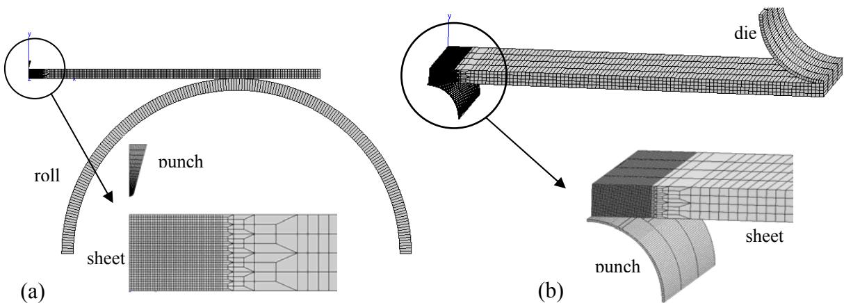
Figure 11: (a) Meshing of the air-bending test, (b) meshing of the stretch bending test.
