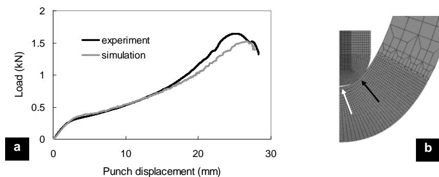
**Figure 12:** (a) Load vs. punch displacement curves for experiment and 2D simulation for a  $180^\circ$  bending angle, (b) The contact area between punch and sheet has moved during the test. Initial contact is illustrated with white arrow and final contact is showed with a black arrow.
