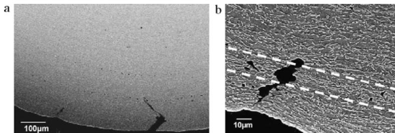
**Fig. 7.** Cross-section SEM observations of sub-surface microcracks of thickness reduced Steel 2 after bending with a 142° angle, case 3 (Nital etching). (a) General view: nucleation and propagation of two microcracks. (b) Close-up view of the bottom left microcrack in (a) which initiated at a hard band (located between white dotted lines). Necking is evidenced between this microcrack and the outer surface.
