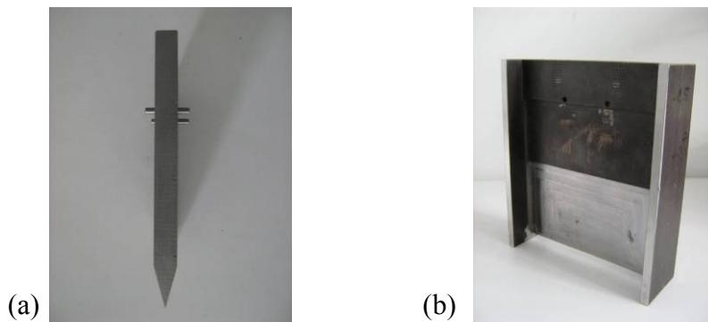
Figure A2.7. Air-bending punches. (a) punch with radius close to 0mm, (b) thin punch with radius of 0.4mm and side stiffeners.
