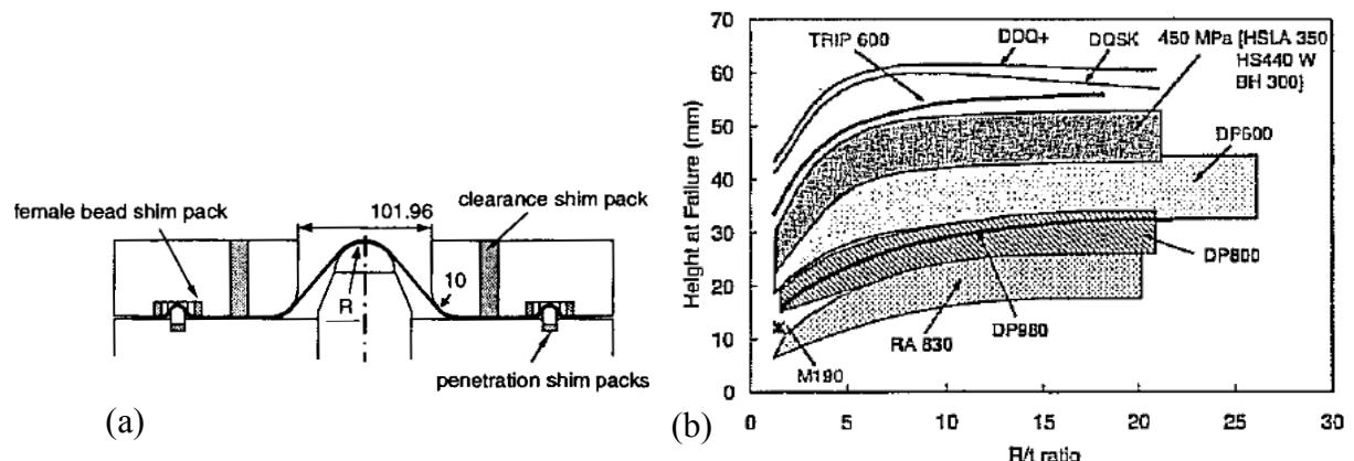
Figure I.11. (a) Stretch bending device, (b) Height at failure as a function of  $R/t$  ratio for structural steels in stretch bending (Sriram et al., 2003).
