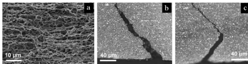
**Fig. 4.** (a) Fractographic observation by SEM after air-bending test of Steel 1. (b and c) Cross-sections of bent specimens of (full-thickness) Steel 1: two types of microcracks are detected at the outer surface. (a) Almost straight microcrack, with some crack deviation (or initiation) at about 50 μm from the outer surface. (b) V-shaped microcrack, possibly initiated at about 70 μm from the outer surface. Optical micrographs, LePera etching.
