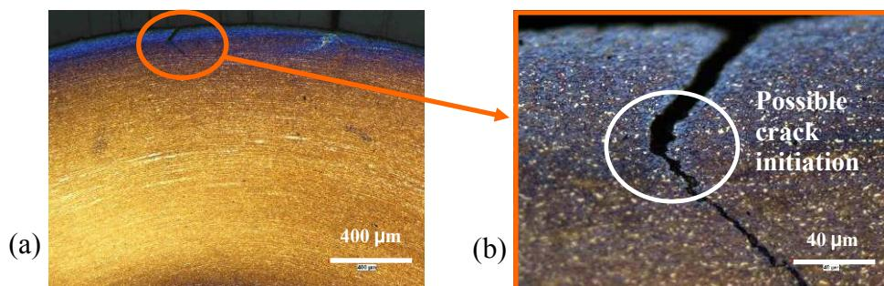
Figure III.9. Cross sectional observations using light microscopy on Steel 1 along the transverse direction, LePera etching. (a) General view, (b) close up view.
