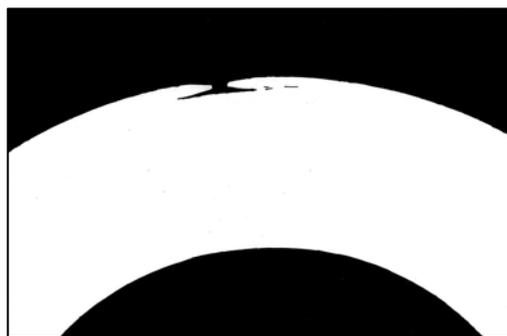
Figure I.3. Crack due to a  $\text{MnS}$  on a wheel rim element (Col, 2010).
