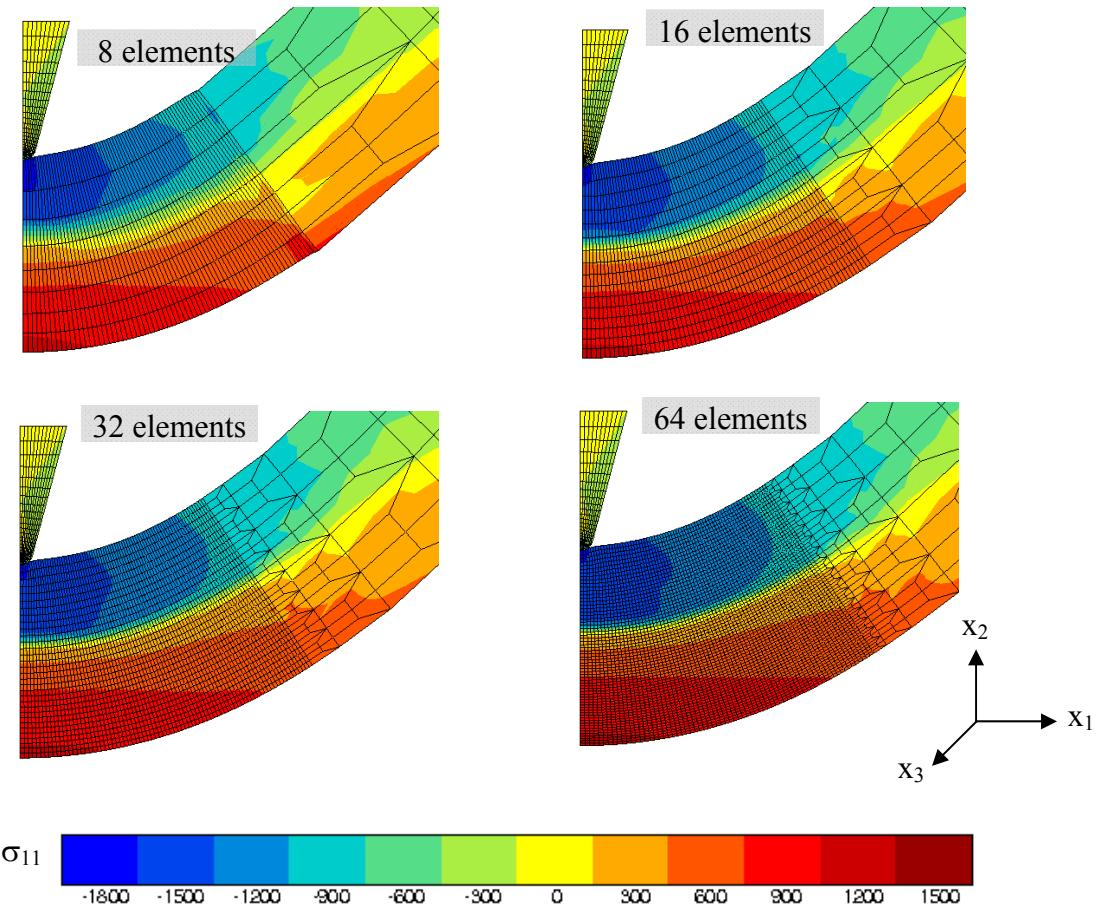
Figure II.12. Stress field after bending of Steel 1.  $\sigma_{11}$  map for the four simulations (8 to 64 elements across the thickness) taken at the end of the test (i.e. for a punch displacement of 26mm).
