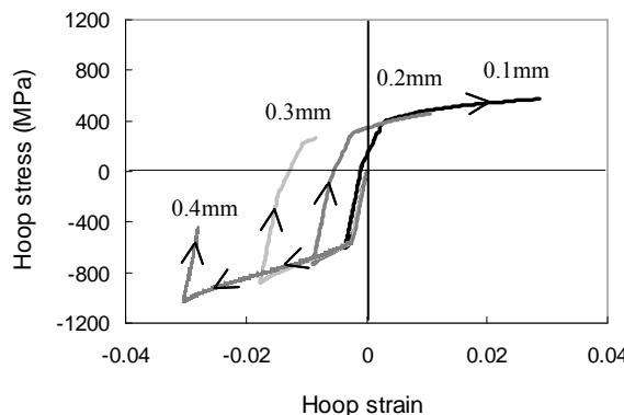
**Figure 10:** Loading paths for various nodes initially next to the mid-thickness, along the symmetry axis. The nodes were initially located at distances from mid-thickness of, respectively, 0.1, 0.2, 0.3, and 0.4mm toward the inner surface.
