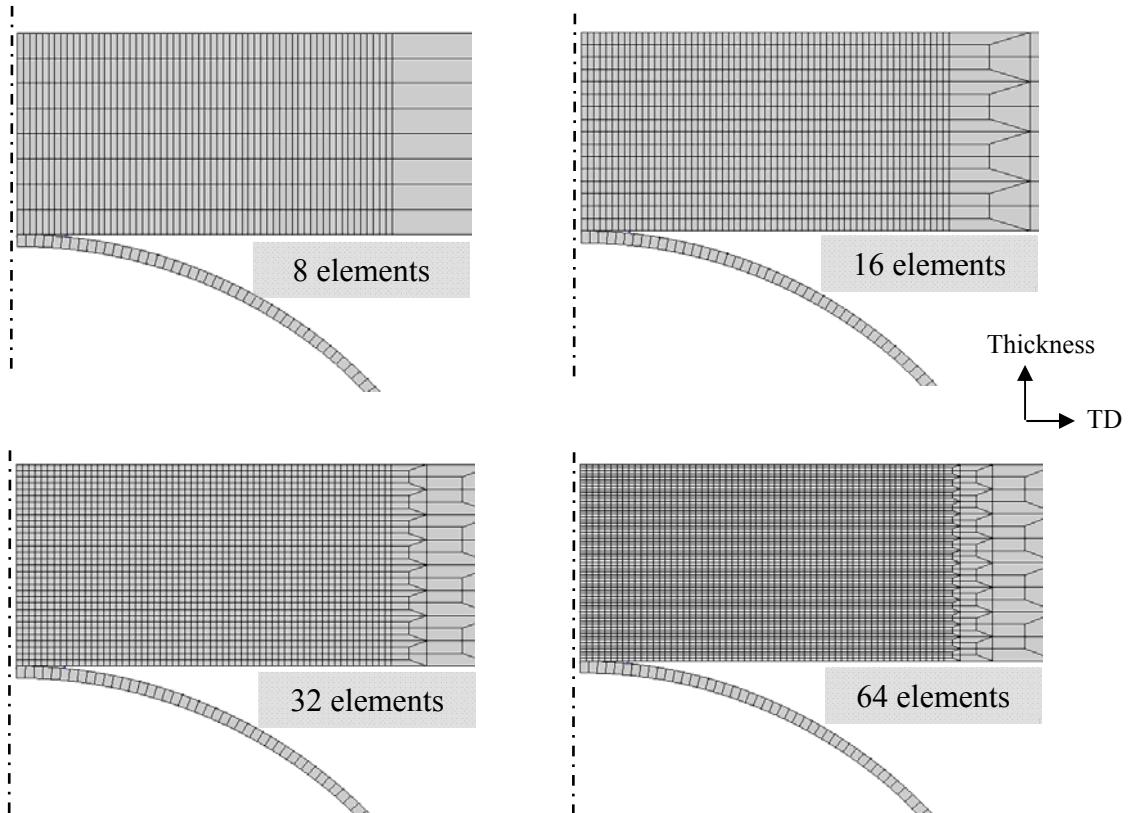
Figure IV.1. Four meshes with various numbers of elements across the thickness. Total thickness = 1.6mm.
