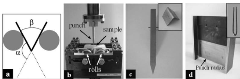
**Fig. 3.** (a) Schematics of air-bending test (with  $\alpha$  the bending angle), bent specimen in black, rolls in grey, punch not represented, (b) air bending device, (c) classical punch with radius = 0.1 mm, bent specimen and (d) thinner punch with radius = 0.4 mm, side stiffeners and thickness-reduced specimen with a bending angle of 180°.
