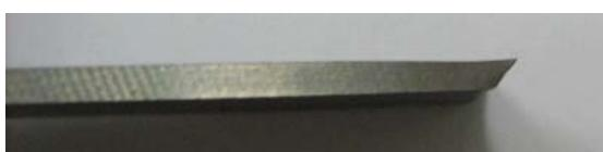
Figure I.34. Broken tensile specimen with a  $45^\circ$  fracture through the thickness.
