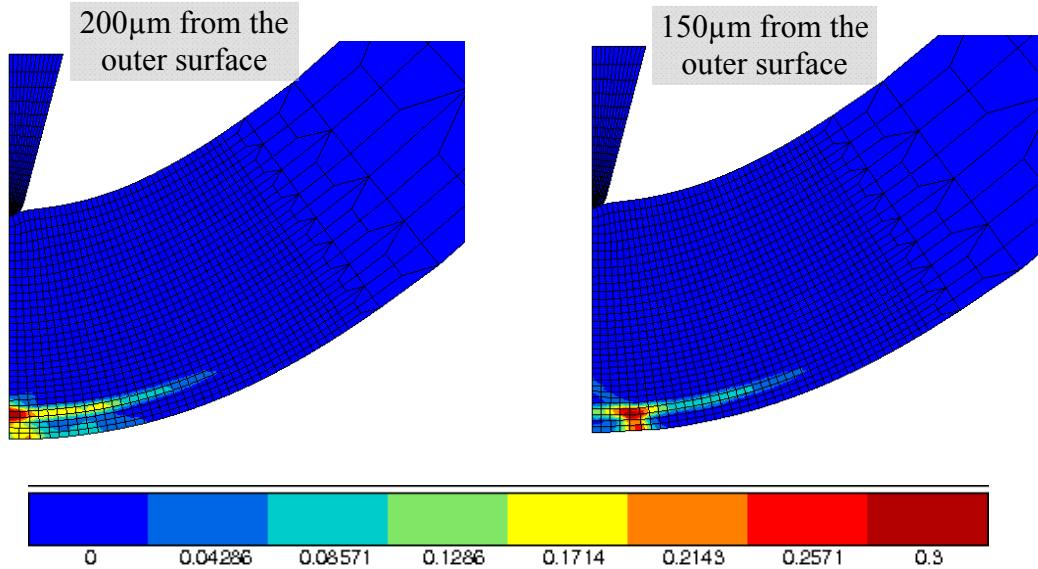
Figure IV.11. Damage map for six initial locations of the band across the thickness. Damage initiates internally as soon as the hard band is initially at 150 $\mu\text{m}$  or less from the outer surface.
