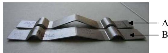
Figure I.38: Picture of two stretch bent samples (A: punch radius = 6mm, B: punch radius = 2mm).
