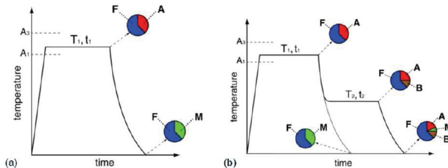
Figure I.14. Heat treatment cycle and microstructures (a) DP steels (b) TRIP steels. F: ferrite; A: austenite; B: bainite; M: martensite (Matsumura et al., 1987).
