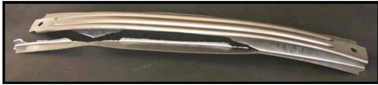
Figure 5. Bumper beam with a large crack along the radius after stamping
