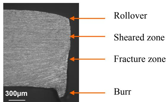
Figure I.1 : Cut edge of a dual phase steel sheet (cross-section micro light optical micrograph) (Dalloz et al., 2007).
