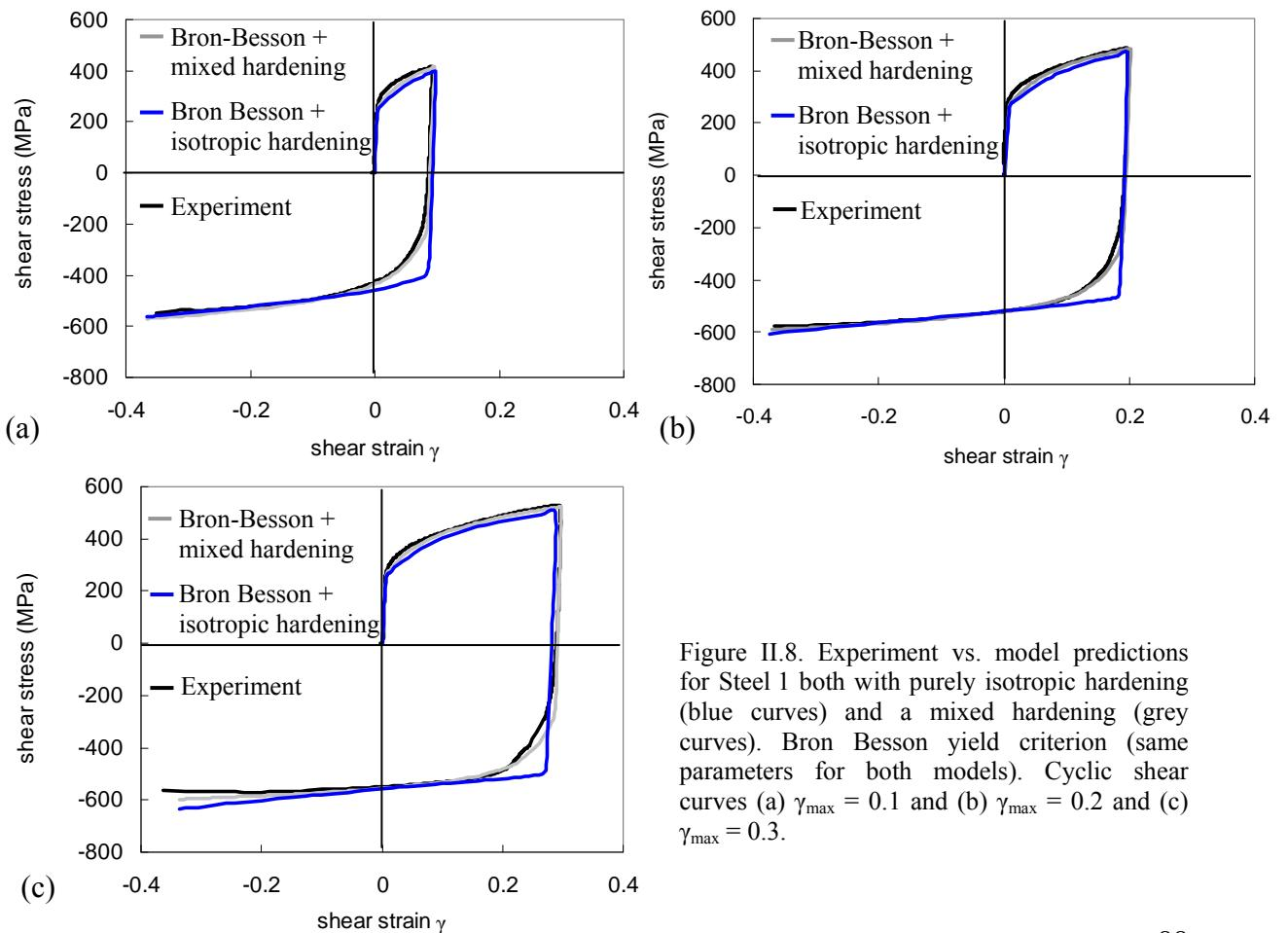
Figure II.8. Experiment vs. model predictions for Steel 1 both with purely isotropic hardening (blue curves) and a mixed hardening (grey curves). Bron Besson yield criterion (same parameters for both models). Cyclic shear curves (a)  $\gamma_{\max} = 0.1$  and (b)  $\gamma_{\max} = 0.2$  and (c)  $\gamma_{\max} = 0.3$ .
