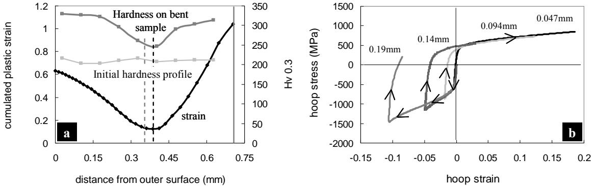
**Figure 14:** (a) Evolution of cumulative plastic strain and hardness through the thickness on a specimen bent up to 180° and initial hardness profile. The neutral fibre shifted from mid-thickness of the sheet toward the inner surface, i.e., the initial compressive zone. The dashed black line and the dashed grey line respectively represent the neutral fibre and the mid-thickness in the updated geometry. The continuous vertical grey line represents the inner surface (thickness reduction).
