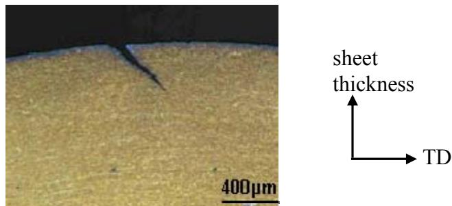
Figure 6: Cross-section of an air-bent specimen. Optical micrograph, LePera etching.
