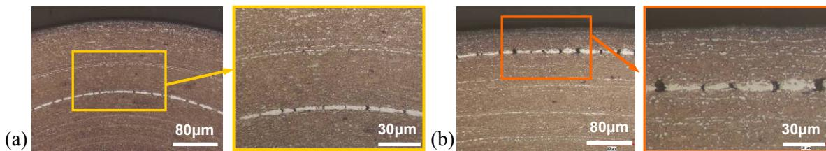
Figure III.27. Optical micrographs of thickness-reduced Steel 2 specimens bent without crack: (a) Segregation 130µm below the surface with a 160° bending angle, (b) segregation 50µm below the surface with a 110° bending angle. Air-bending along TD.
