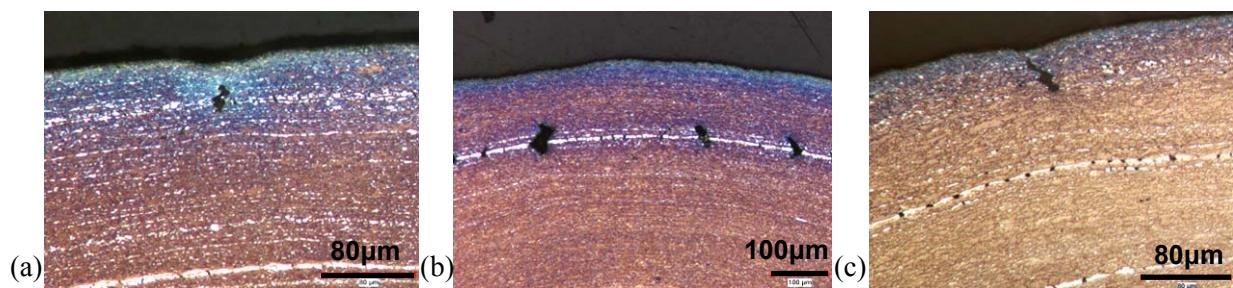
Figure III.28. Optical micrographs of sub-surface cracks for three air-bent thickness-reduced Steel 2 specimens with a 142° angle (LePera etching).
