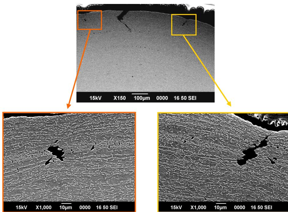
Figure III.30. SEM observations of sub-surface cracks of two thickness-reduced Steel 2 bent specimens (Nital etching), 142° bending angle.
