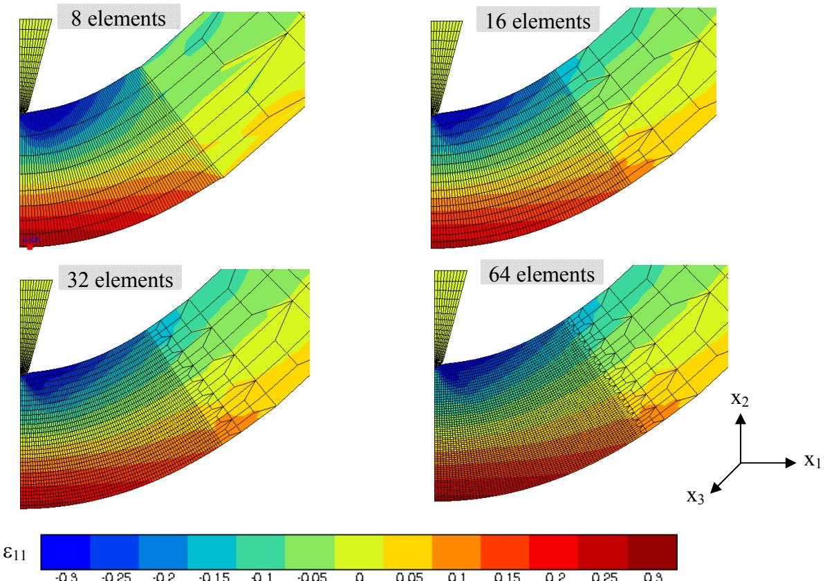
Figure II.11. Strain field after bending of Steel 1.  $\varepsilon_{11}$  map for the four simulations (8 to 64 elements across the thickness) taken at the end of the test (i.e. for a punch displacement of 26mm).
