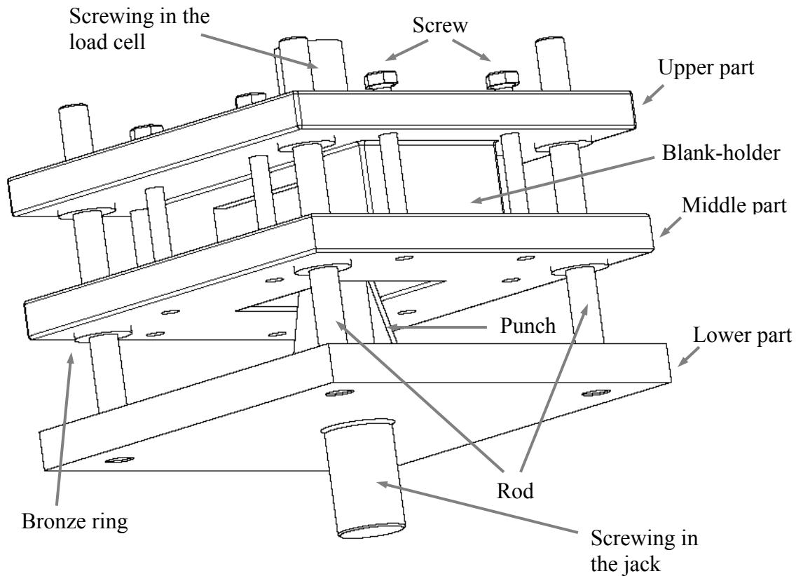
Figure A2.12. General view of the stretch bending device.
