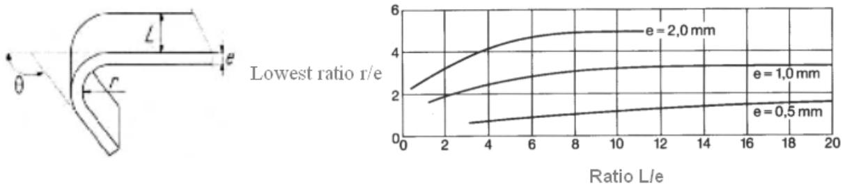
Figure I.2: Minimum bending radius evolution according to sample width for copper alloys (CuFe<sub>2</sub>P) with various values of thickness (Determe, 1998).
