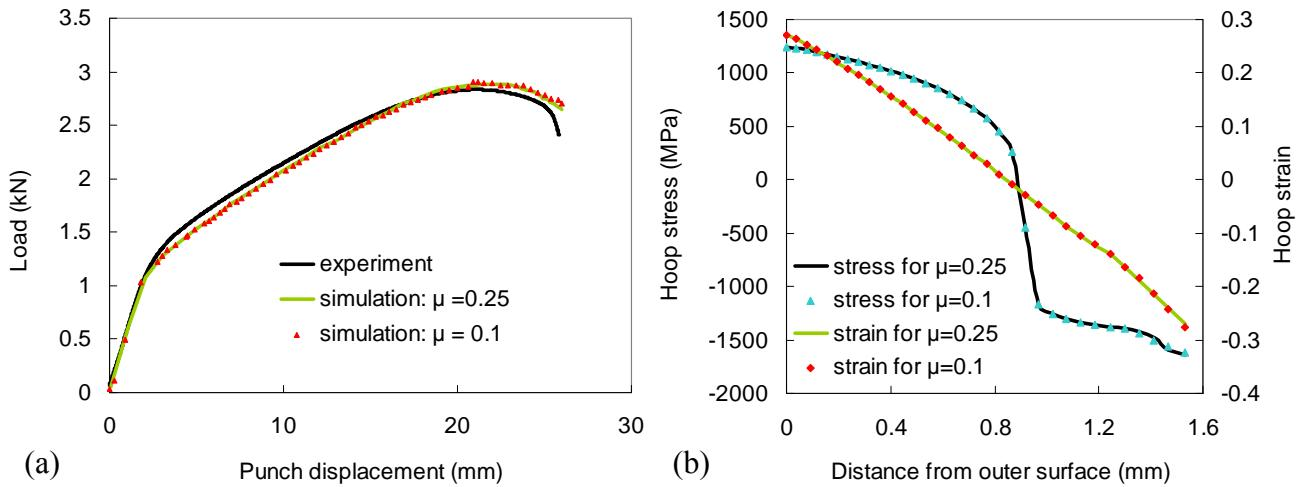
Figure II.13. Influence of the friction coefficient on the air-bending test with  $\mu = 0.25$  and  $\mu = 0.1$  (a) experimental and predicted load / displacement curves, (b) hoop stress and hoop strain distributions for both friction coefficients at the end of the test (i.e. a punch displacement of 26mm).
