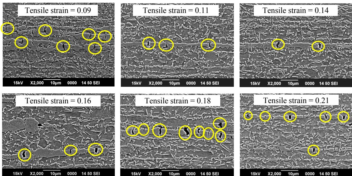
Figure III.21. Damage development during uniaxial tension of Steel 3 - various tensile true strain levels (from 0.09 up to 0.21) (Nital etching).
