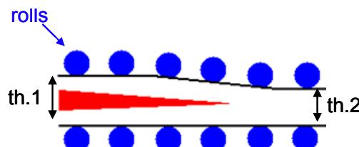
Figure I.23: Soft reduction principle from thickness th.1 down to thickness th.2 at the end of the solidification.
