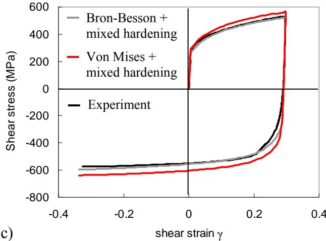
Figure II.5. Experiment vs. model predictions for Steel 1 both with a Von Mises (red curves) and a Bron Besson (grey curves) yield criterion. Mixed isotropic/kinematic hardening rule. Cyclic shearing curves (a)  $\gamma_{\max} = 0.1$  and (b)  $\gamma_{\max} = 0.2$  and (c)  $\gamma_{\max} = 0.3$ .
