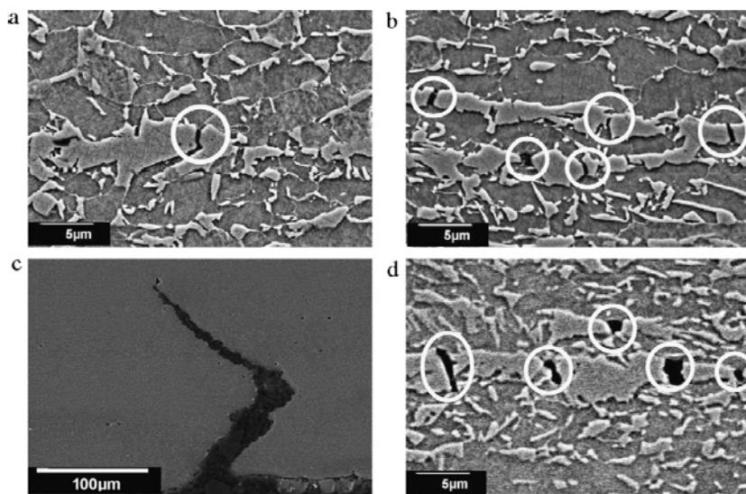
**Fig. 5.** (a and b) SEM observations of damage after interrupted uniaxial tensile tests of Steel 1 (Nital etching). Cavities (in white circles) are observed at hard bands. Average axial strain = 0.11 for (a) and 0.17 for (b). (c and d) SEM observations of damage after air-bending. (c) General view of a bending crack and (d) damage development at hard bands close to the outer surface (Steel 2, case 3).
