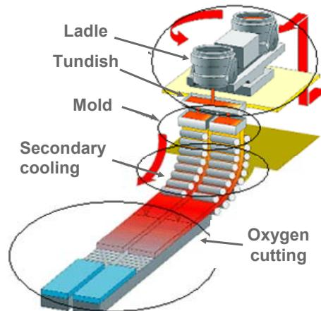
Figure I.17: Continuous casting.
