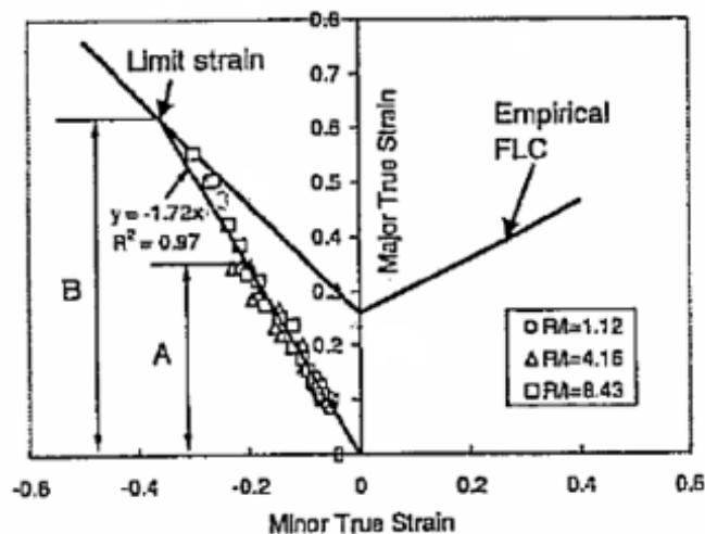
Figure I.6. Strain path and stretch bendability index (SBI) for 0.93mm BH210 specimens (Sriram et al., 2003).
