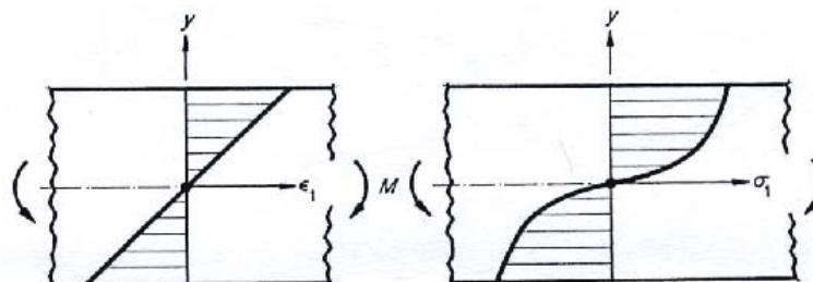
Figure I.13: Strain and stress distribution for a material in pure bending that obeys the relation  $\sigma_1 = k\epsilon_1^n$  (Marciniak and Duncan, 1992).
