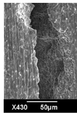
Figure III.2. Ductile failure of Steel 1 after air-bending.
