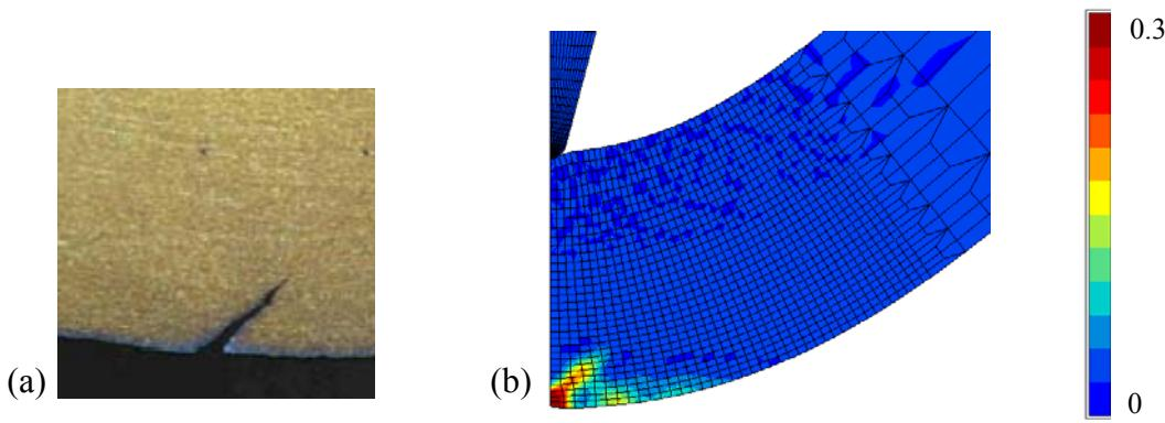
Figure 14: (a) crack on an air-bent specimen, (b) damage map at the end of the air-bending test.
