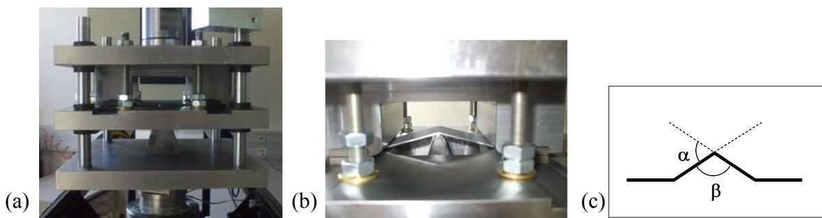
Figure 3: (a) stretch bending device, (b) stretch bending test in progress with specimen clamped between die and blank-holder and a punch radius of 4mm, (c) schematics of the stretch bent sheet (thick line) with  $\alpha$  = bending angle.
