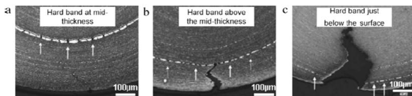
**Fig. 6.** Cross-section optical micrographs (LePera etching) after a 180° bending of thickness-reduced Steel 2. (a) Case 2, (b) case 3 and (c) case 4. White lines are thicker hard bands.
