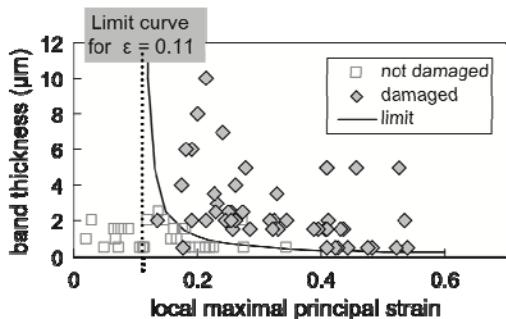
**Fig. 9.** Damage development criterion (Eq. (3)) at hard bands for all bent specimens (observed from 2D sections) as a function of the local band thickness and the local "mesoscopic" maximal principal strain calculated with the analytical formula.
