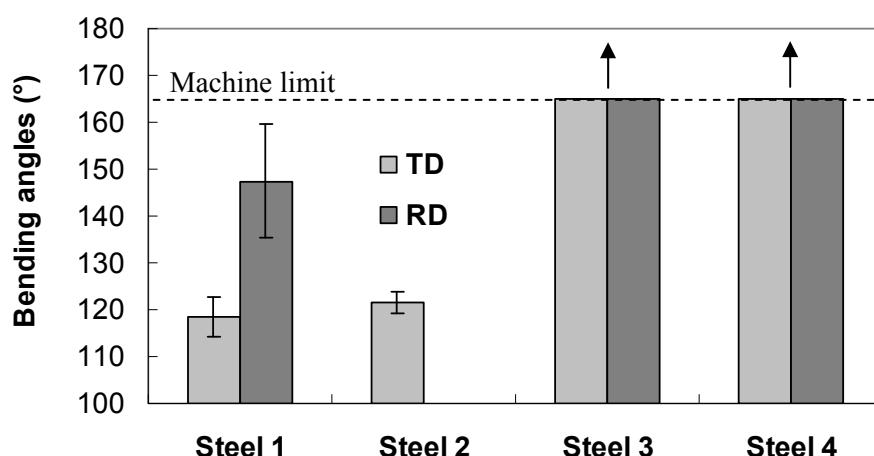
Figure I.36. Air-bending results for each TRIP steel.
