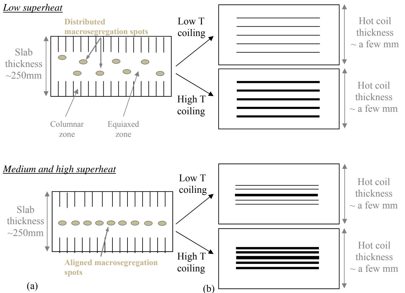
Figure I.24: (a) Superheat effect on the slab structure before hot rolling and (b) temperature coiling effect on the banded structures after hot rolling.
