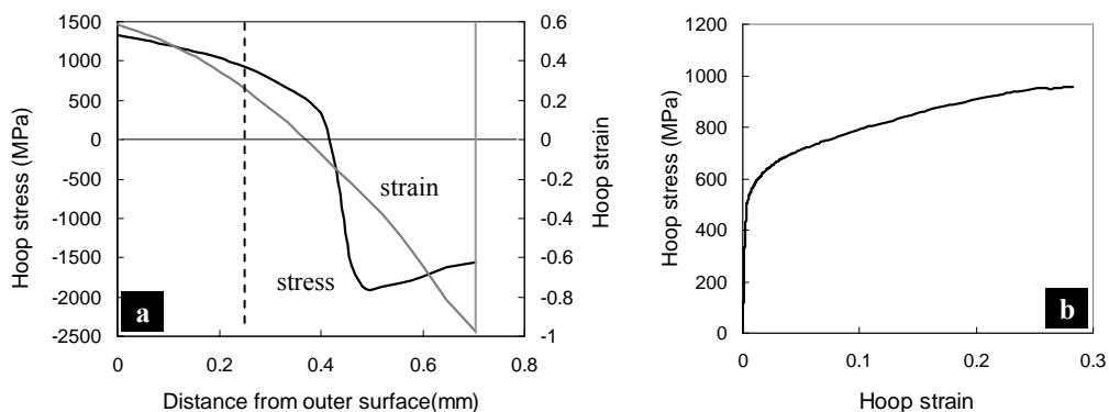
**Figure 15:** (a) Hoop stress (black line) and hoop strain (grey line) along the symmetry axis for a 180° bending (thickness-reduced Steel 2). The location of material initially at mid-thickness is represented by the vertical dashed line (0.23mm from outer surface). The inner surface is represented by the vertical grey line (thickness reduction), (b) hoop stress vs. hoop strain evolution for the node initially at mid-thickness.
