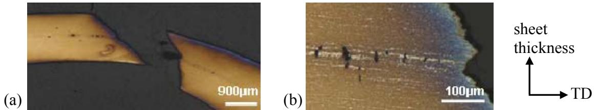
Figure 7: Optical micrographs after stretch bending. LePera etching. (a) General view of a broken sample, (b) close-up view of damage close to the central hard band.
