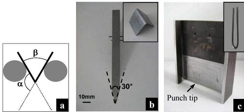
**Figure 1:** (a) schematics of the air-bending test with  $\alpha$  = bending angle, (b) punch with radius = 0.1mm, punch thickness = 10mm and (inlet) a bent sample, (c) thin punch with side stiffeners and radius = 0.4mm, punch thickness = 0.8mm and (inlet) a 180° bent sample.
