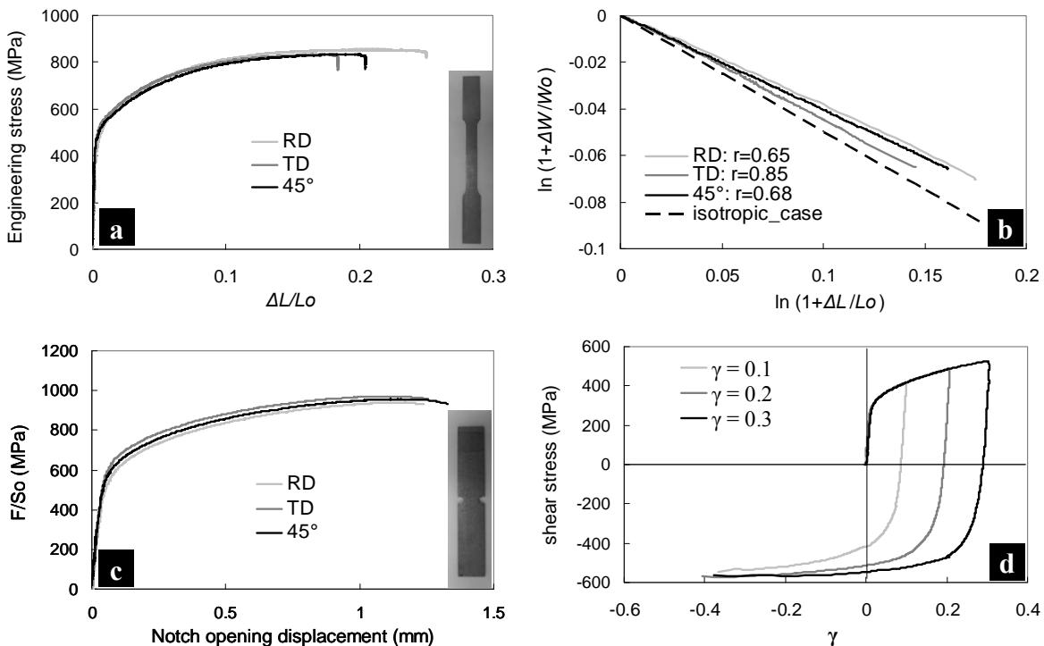
**Figure 2:** (a) Engineering tensile stress-strain curves, (b) strain anisotropy (smooth tensile specimens), (c) Tensile curves on NT specimens where F is the load and  $S_0$  is the initial cross section between notch roots, (d) cyclic shear curves along RD.  $\gamma$  corresponds to the ratio between the horizontal displacement and the specimen width = 4.5mm.
