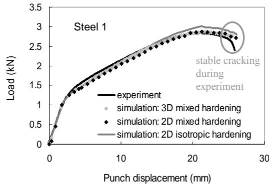
Figure 6: Experimental and predicted load vs. displacement curves both in 2D and 3D with a mixed isotropic/kinematic hardening rule (boundary condition (ii)) and in 2D with an isotropic hardening rule (boundary condition (i)).
