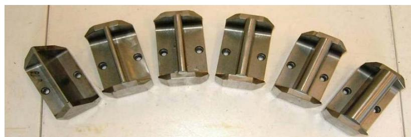
Figure A2.10. Various punches ( $R = 2$  to 15 mm).
