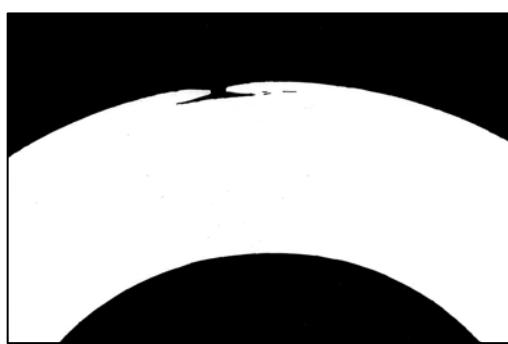
Figure I.3. Crack due to a MnS on a wheel rim element (Col, 2010).
