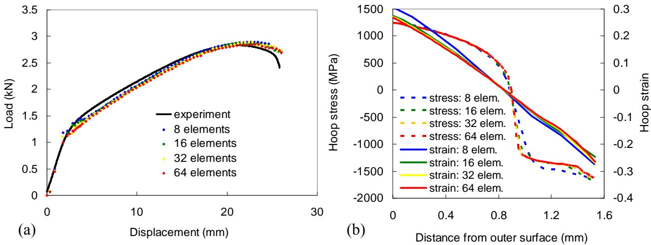
Figure II.10. (a) Influence of the mesh on the load / displacement curves. Calculations with the Bron Besson yield criterion, mixed isotropic/kinematic hardening rules. (b) Influence of the mesh on the hoop stress and hoop strain distributions across the thickness at the end of the test (i.e. for a punch displacement of 26mm).
