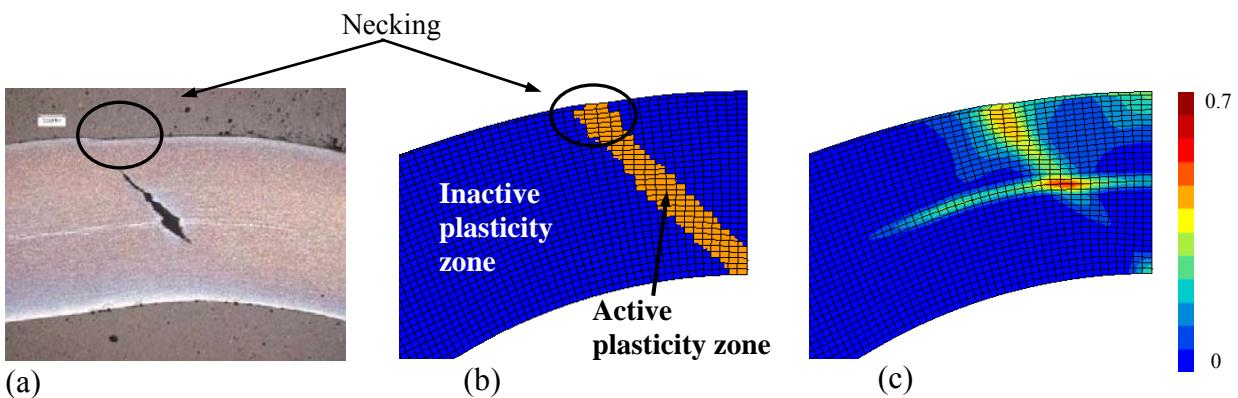
Figure 16: (a) cross-sectional observation of an internal crack during stretch bending (b) active and inactive plasticity zones: localization within a  $45^\circ$  band and (c) damage map taken at mid-width for a punch displacement of 22mm.
