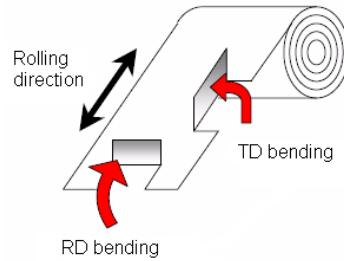
Figure I.4 : Bend orientation with respect to the coil (Determe, 1998).
