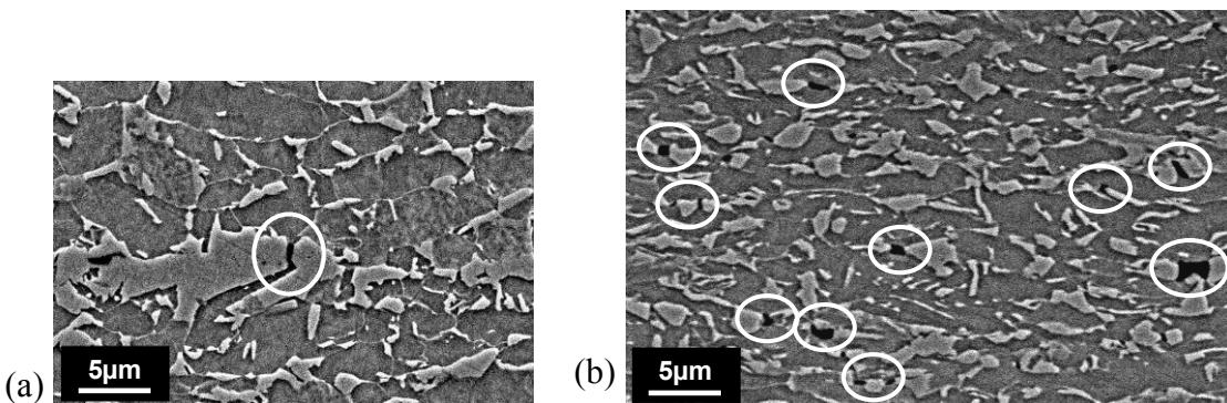
Figure 10: cross-section SEM observations of damage after a Nital etching. Damage cavities are surrounded with white circles. (a) Damage at hard band after an interrupted uniaxial tensile test ( $\epsilon = 0.11$ ), (b) damage in the softer matrix with either decohesion at martensite/ferrite interface or with cleavage at martensite islands (air-bent specimen).
