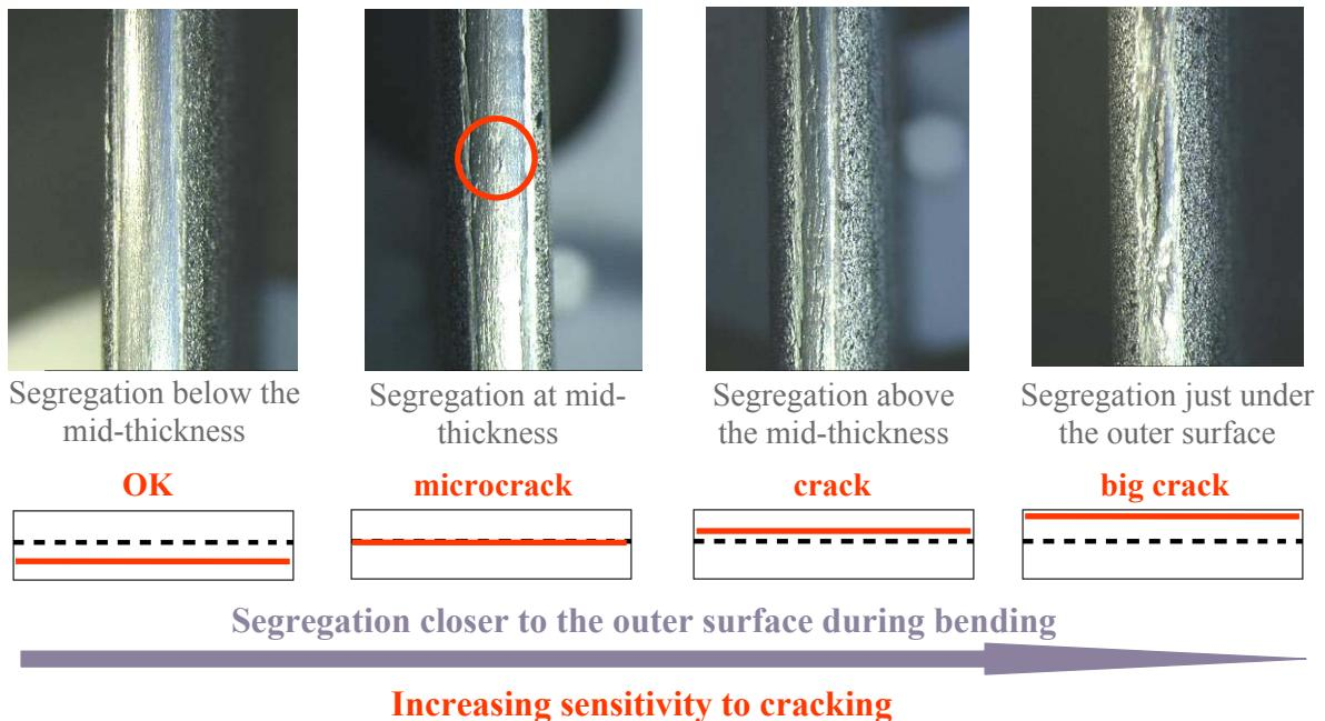
Figure III.25. Macrographic observations of four specimens of reduced-thickness Steel 2 bent along TD up to  $180^\circ$  with various locations of the main segregation band.
