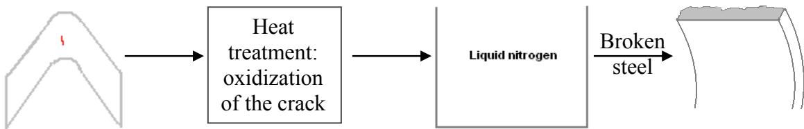
Figure III.3. Steps to mark the crack by oxidization.
