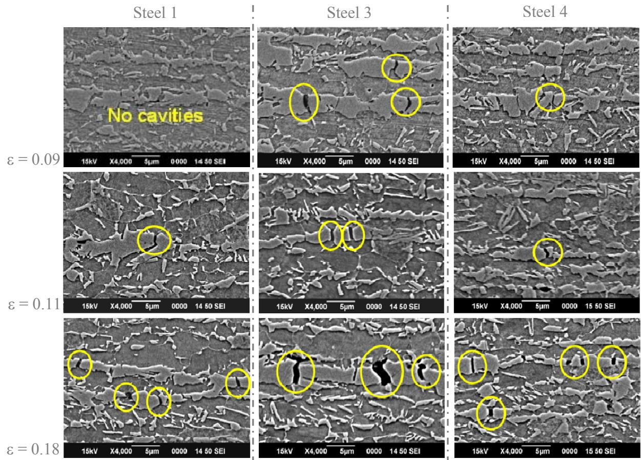
Figure III.20. SEM observations after Nital etching of the three TRIP steels (1.6mm in thickness) after a uniaxial tensile true strain of 0.09, 0.11 and 0.18.”
