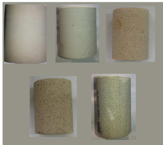
Figure 56: Cores corresponding to the 5 porous media analyzed in this study. From left to right in the first row: a) A10 sintered silicate; b) less permeable and porous A10 sintered silicate; c) Bentheimer sandstone; d) Castlegate sandstone; e) Berea sandstone.
