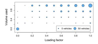
Figure 4.5: Loading factor and volume used in 5 axle vehicles
