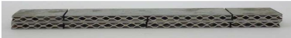
Fig. 2.6 : Shear-lap test experiment specimen.
