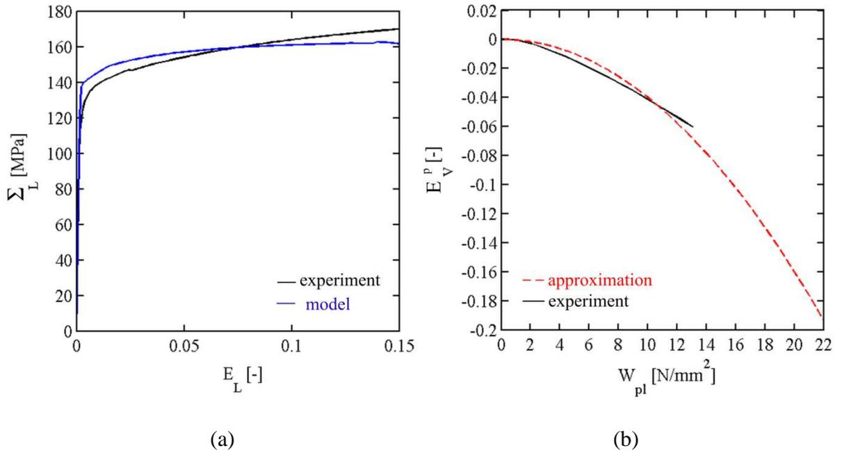
Figure 4.2 : (a) Stress-strain curves for the uniaxial tensile experiment (in black the “virtual” experiment results, in blue the model results) along with (b) the plastic volume change as a function of the plastic work density.
