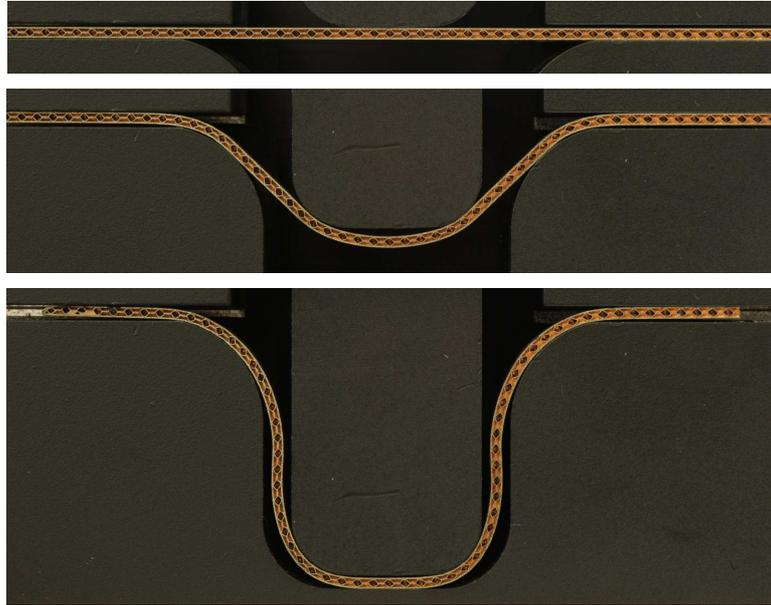
Figure 4.6 : Draw bending of a prototype sandwich sheet demonstrating the formability of the sandwich sheet material.
