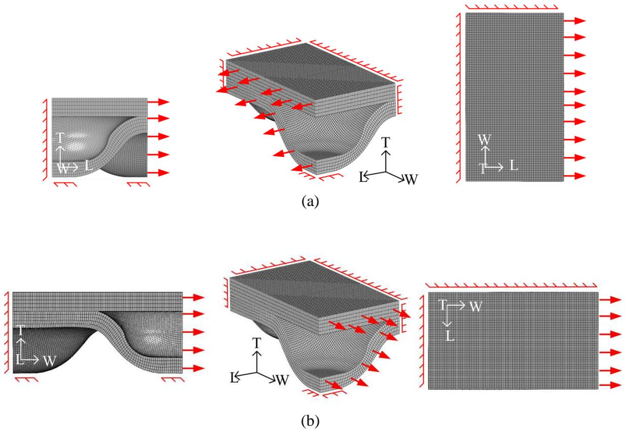
Fig. 3.2 : Illustration of the displacement boundary conditions for uniaxial tension (a) in the L-direction and (b) in the W-direction.
