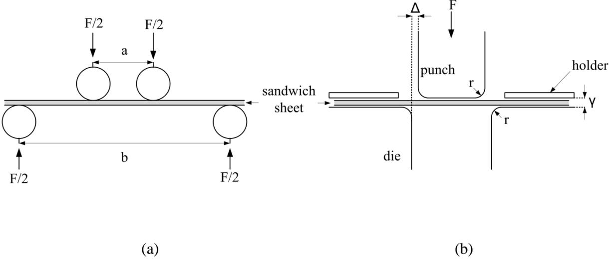
Figure 4.1 : Technical drawing of the experimental set-ups: (a) four-point bending experiment, (b) draw bending experiment.
