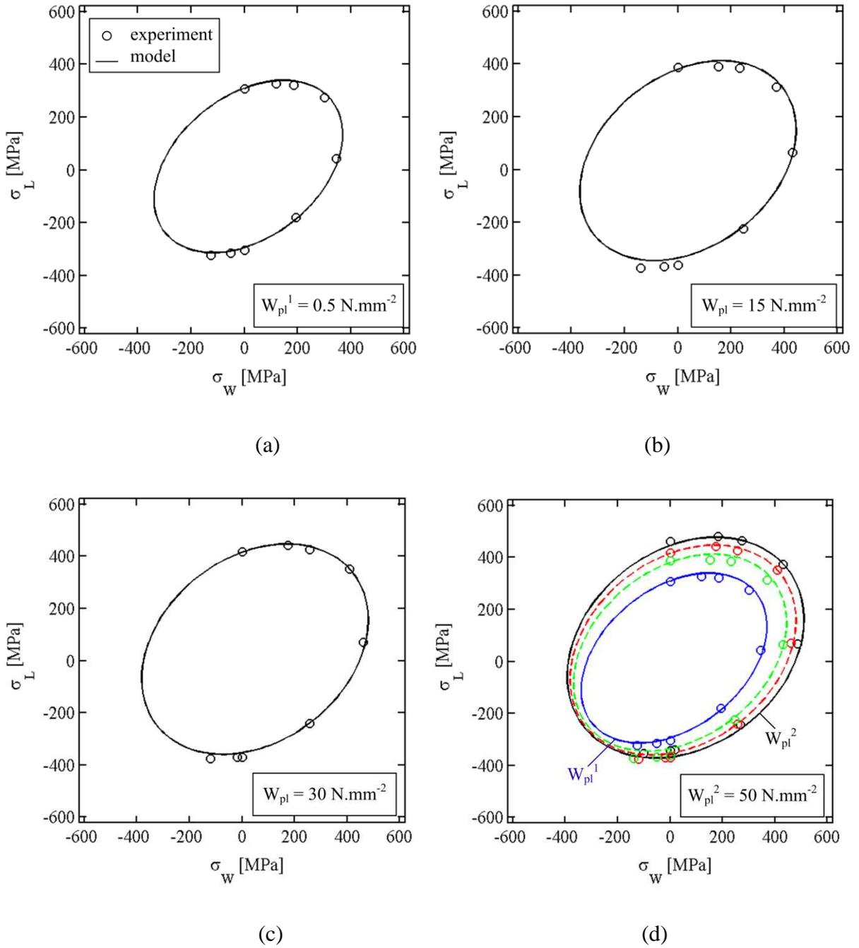
Fig. 3.10 : Envelopes of equal plastic work (per unit initial volume) for the face sheets in the true stress plane ( $\sigma_W, \sigma_L$ ). The open dots present the results from virtual experiments, the black solid lines in (a) and (d) represent the least square fit of the yield function given by Eq. (3.16). The solid envelopes in (b) and (c) have been computed based on the isotropic-distortional hardening model given by Eq. (3.24).
