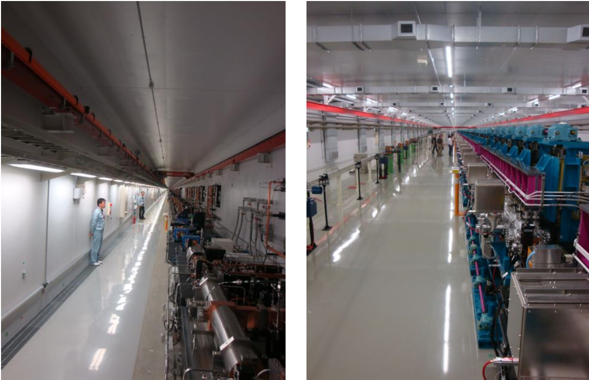
Figure 5.4: The accelerator (left) and magnetic undulator (right) of the free-electron laser SACLA, during a visit organized for the FEL2012 conference.
