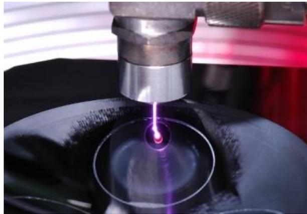
Fig. 25 Ion and plasma beam machining from TNO.
