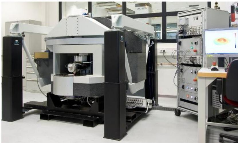
Fig. 39 NANOMEFOS non-contact measurement machine for freeform optics [2].
