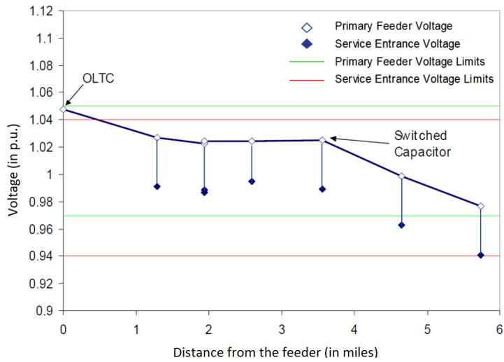
Figure 17: Voltage in a distribution without DG, source: [5]
