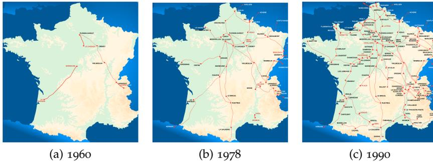
Figure 4: Evolution of the high-voltage (400 kV) network in France, source : RTE
