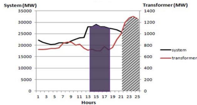
Figure 25: Use of storage in combination with intermittent and inflexible generators, source: NRStor
