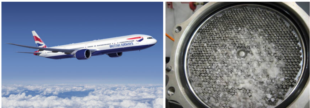
Figure 1 – Ice on the inlet face of a fuel-oil heat exchanger similar to that of BA38 Boeing 777.
